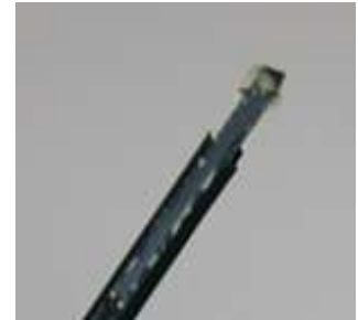
EX3DV4 E-Field Probe
