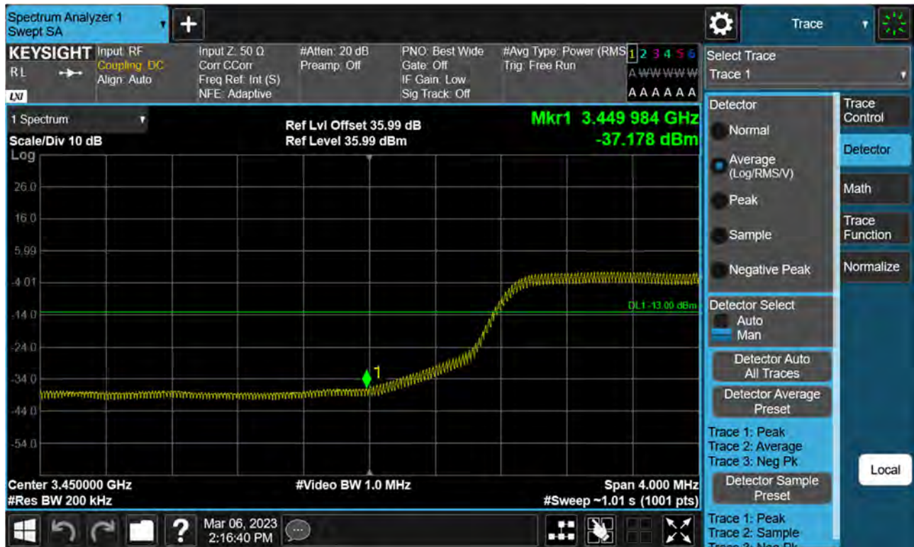
Sub6 n77(78). Low Band Edge Plot (90 M BW Ch.633000 BPSK FullRB)(1)
