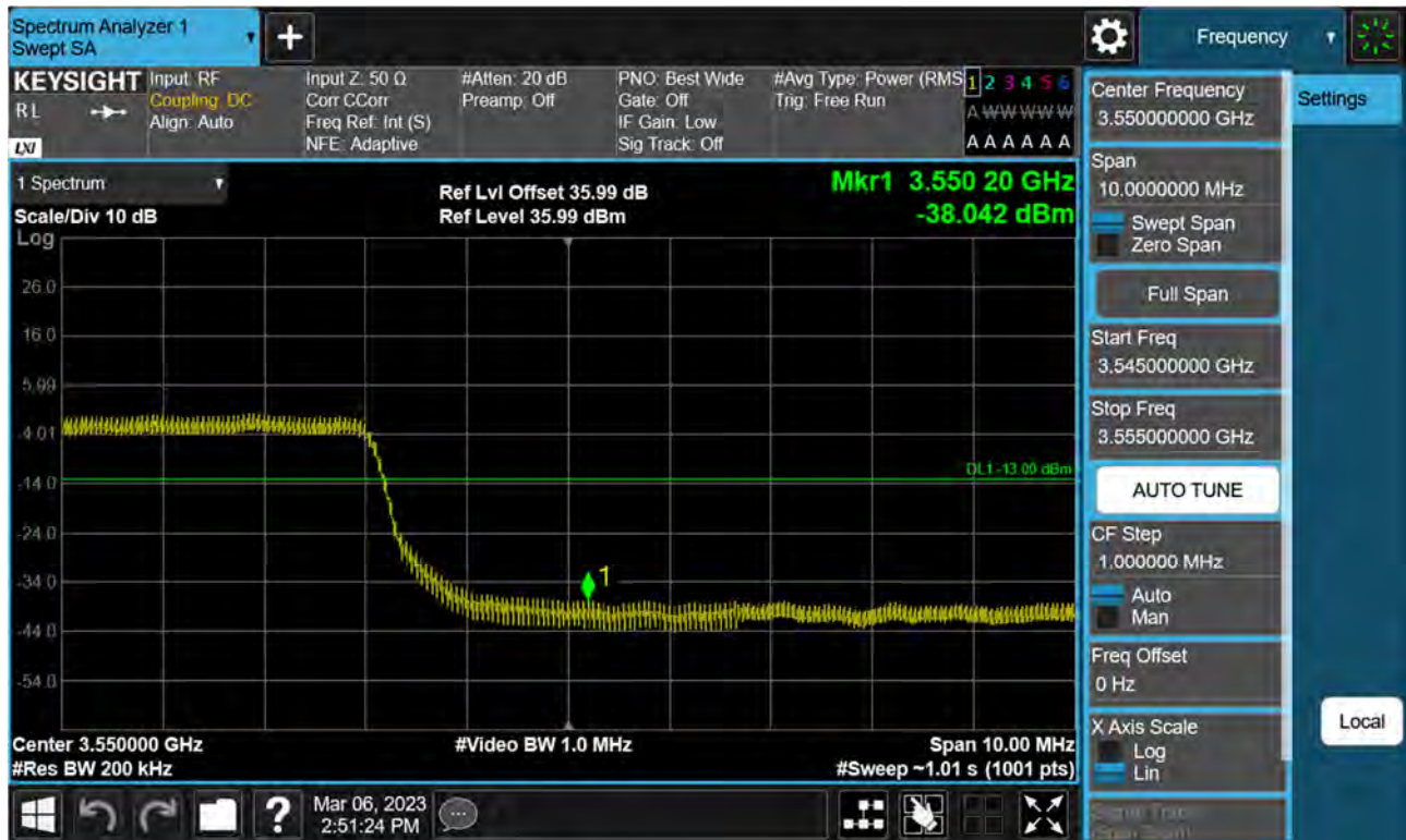
Sub6 n77(78). High Band Edge Plot (100 M BW Ch.633334 BPSK FullRB)(1)
