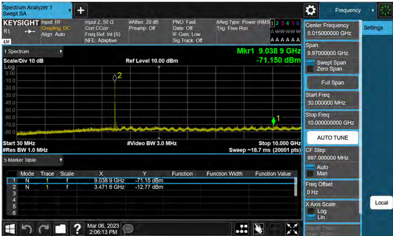
Sub6 n77(78). Conducted Spurious Plot_1 (634000ch_80 MHz_BPSK)
