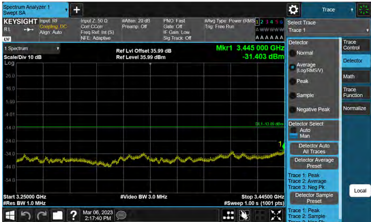
Sub6 n77(78). Low Band Edge Plot (90 M BW Ch.633000 BPSK FullRB)(3)
