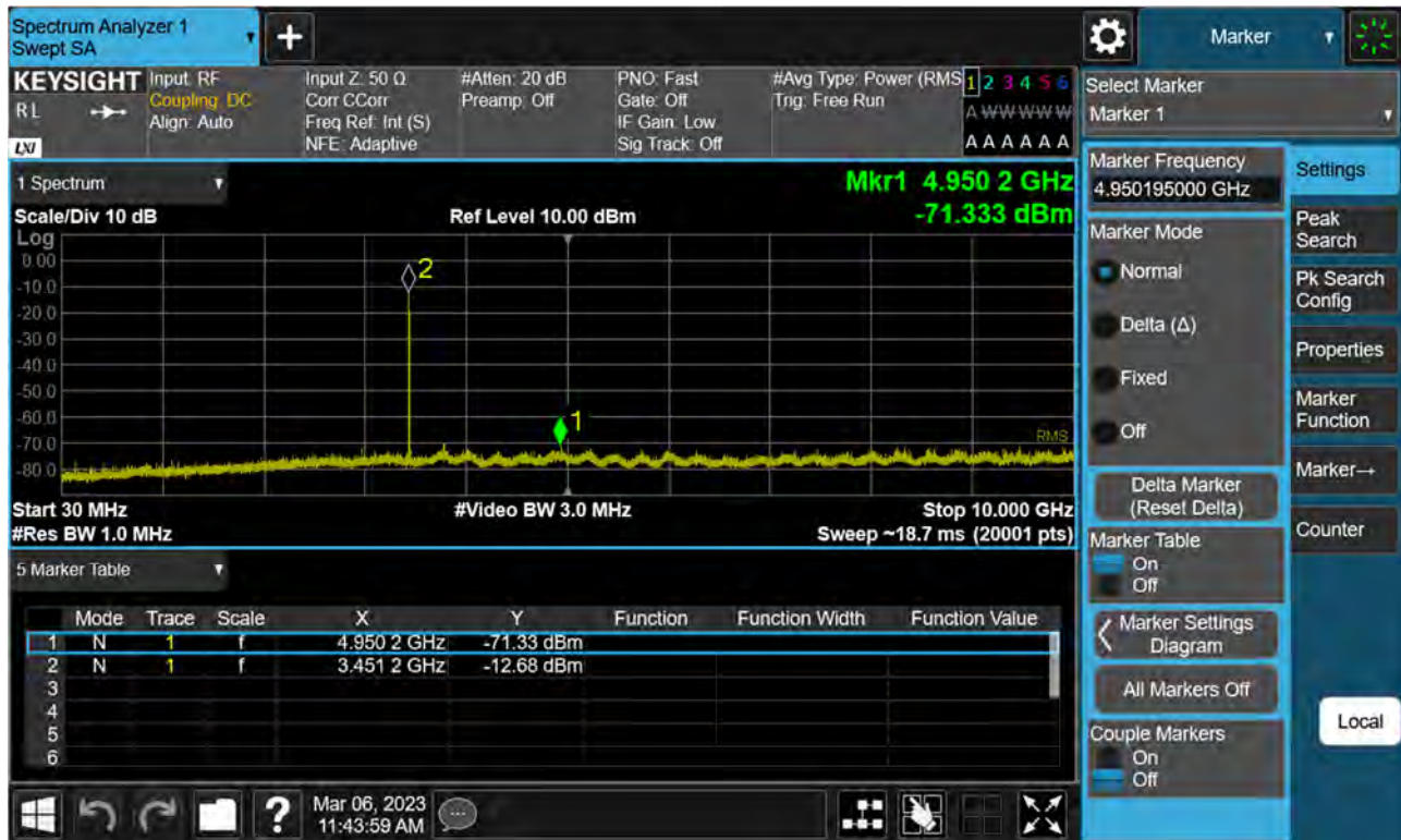
Sub6 n77(78). Conducted Spurious Plot_1 (630668ch_20 MHz_BPSK)
