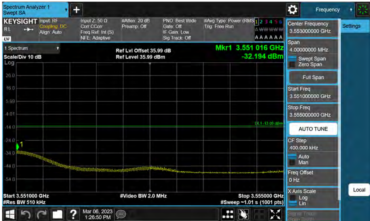
Sub6 n77(78). High Band Edge Plot (60 M BW Ch.634666 BPSK 1RB)(2)
