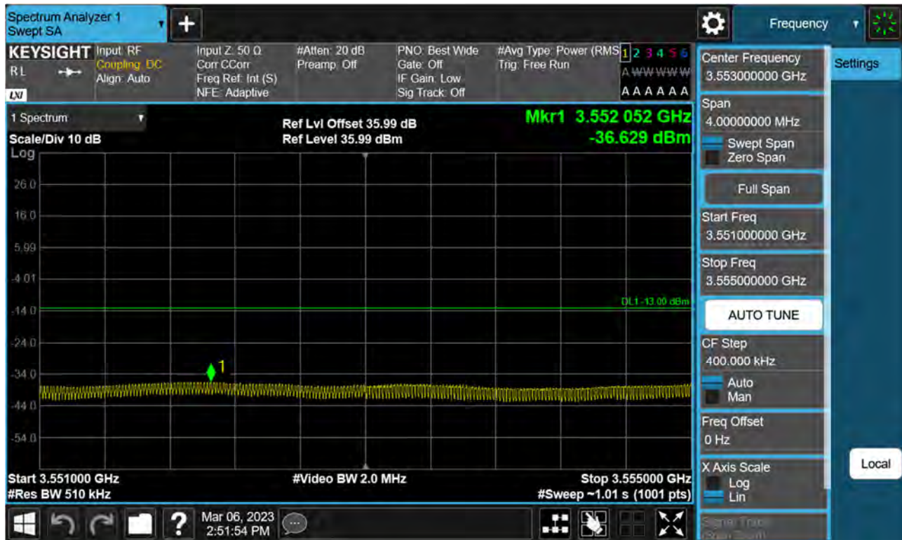
Sub6 n77(78). High Band Edge Plot (100 M BW Ch.633334 BPSK FullRB)(2)
