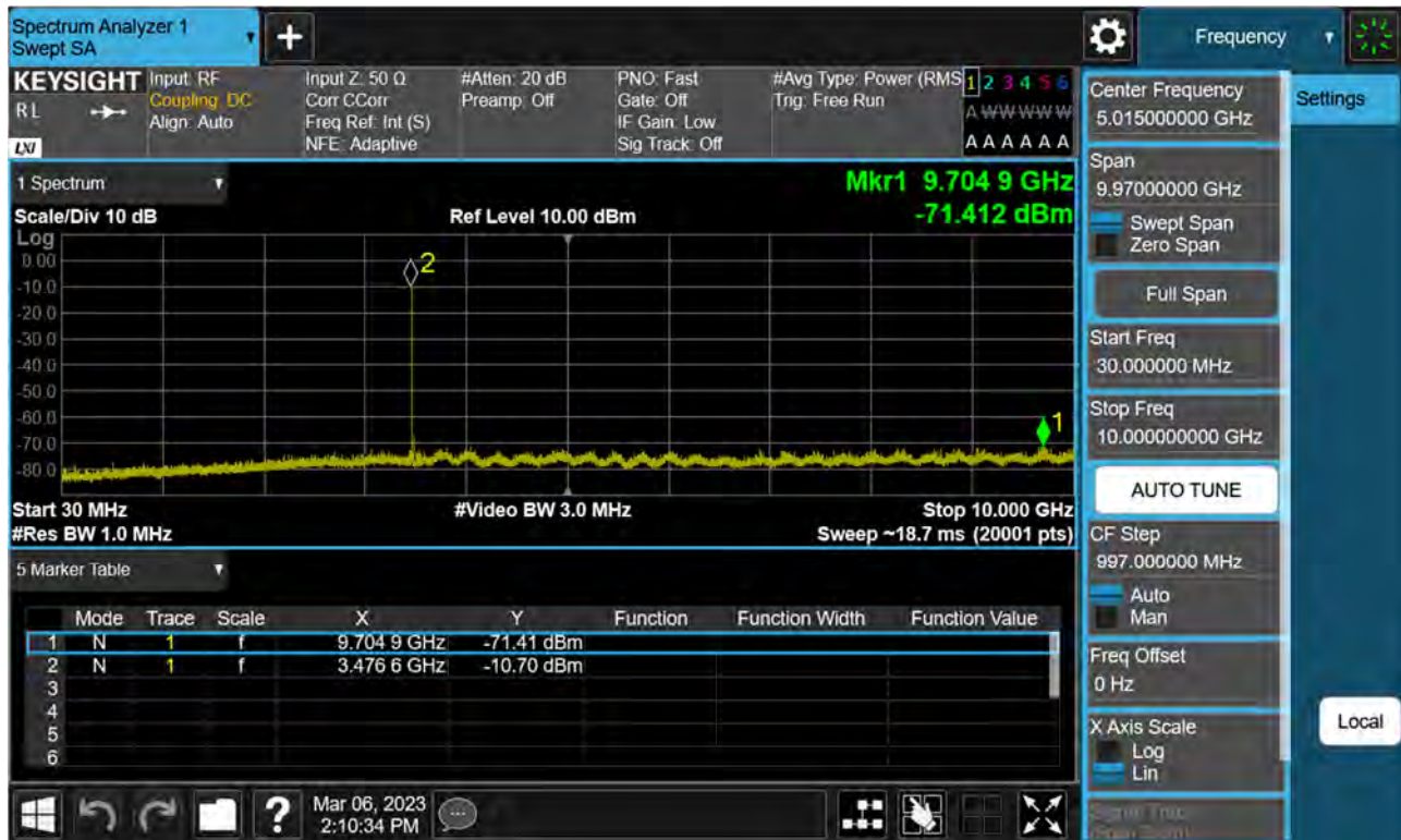
Sub6 n77(78). Conducted Spurious Plot_1 (633334ch_50 MHz_BPSK)
