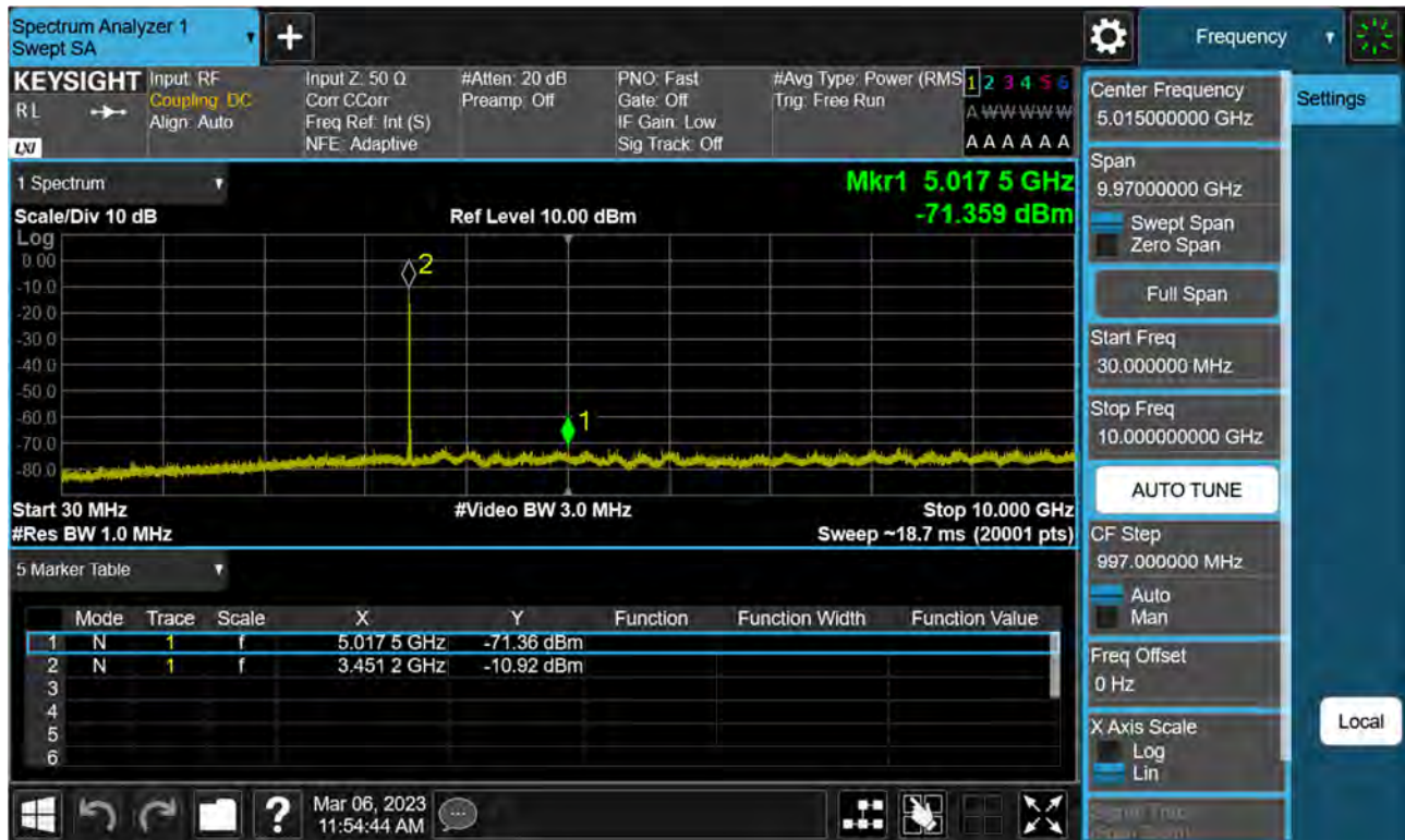
Sub6 n77(78). Conducted Spurious Plot_1 (631000ch_30 MHz_BPSK)
