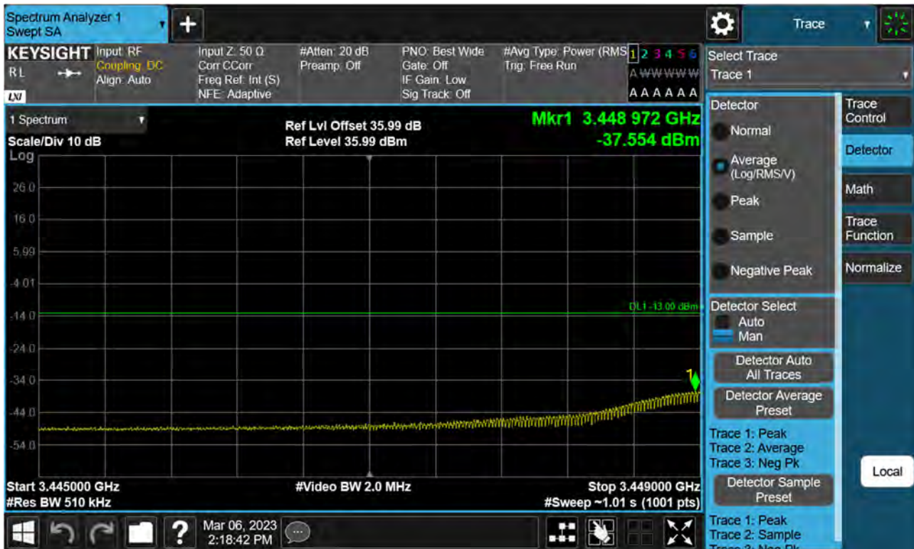
Sub6 n77(78). Low Band Edge Plot (90 M BW Ch.633000 BPSK 1RB)(2)
