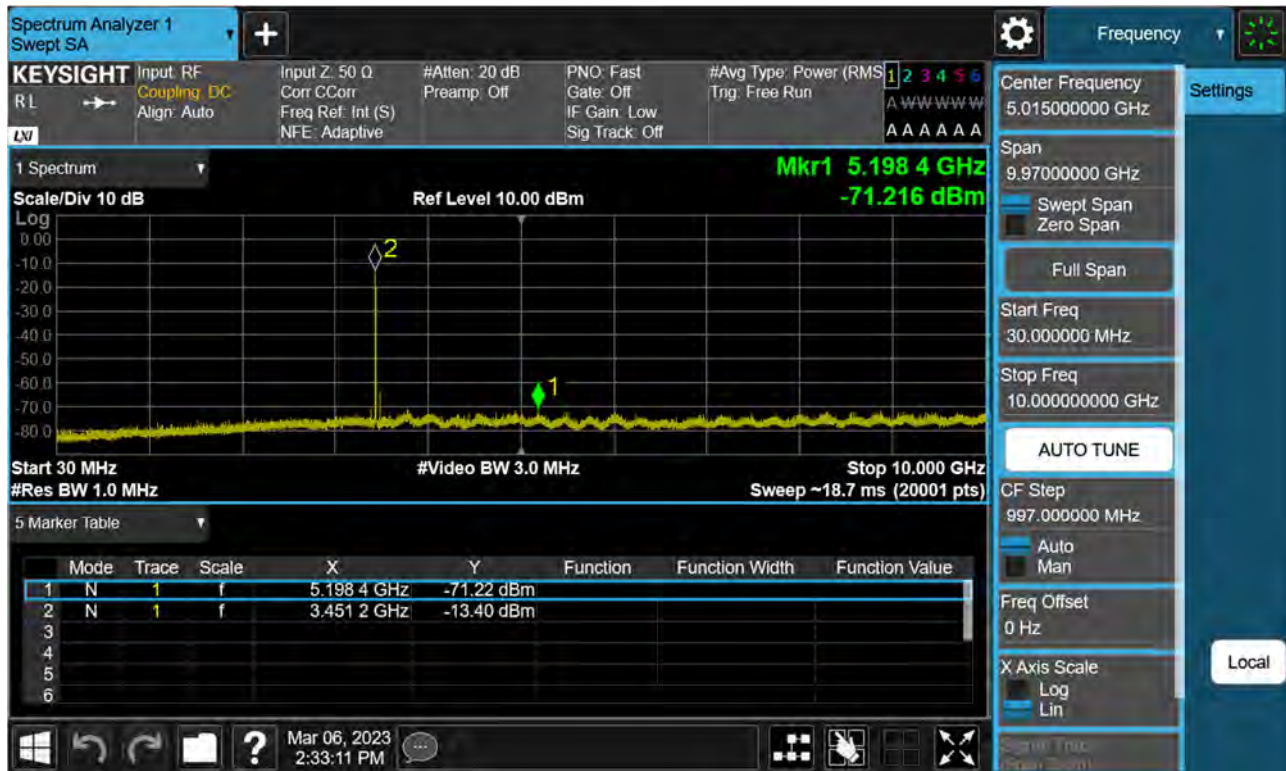
Sub6 n77(78). Conducted Spurious Plot_1 (633334ch_100 MHz_BPSK)
