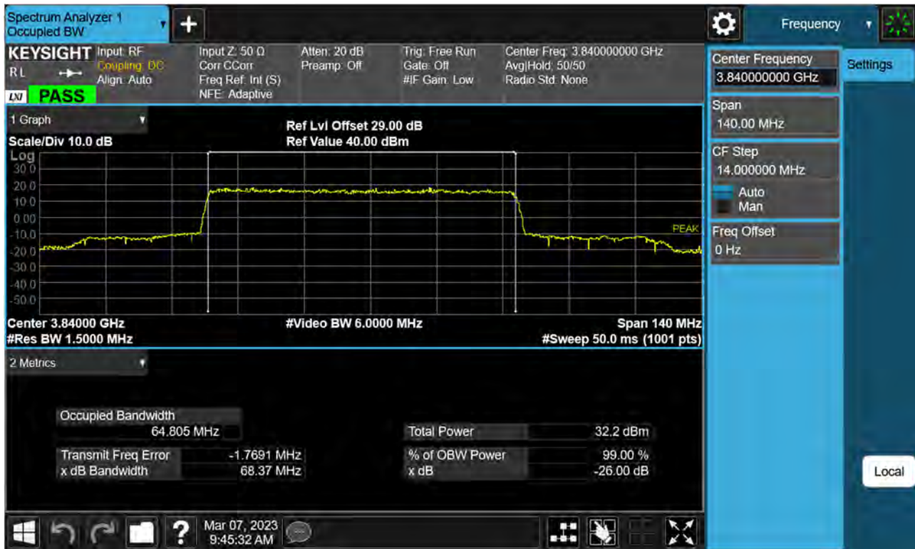
Sub6 n77(78). Occupied Bandwidth Plot (70 M BW Ch.656000 QPSK)
