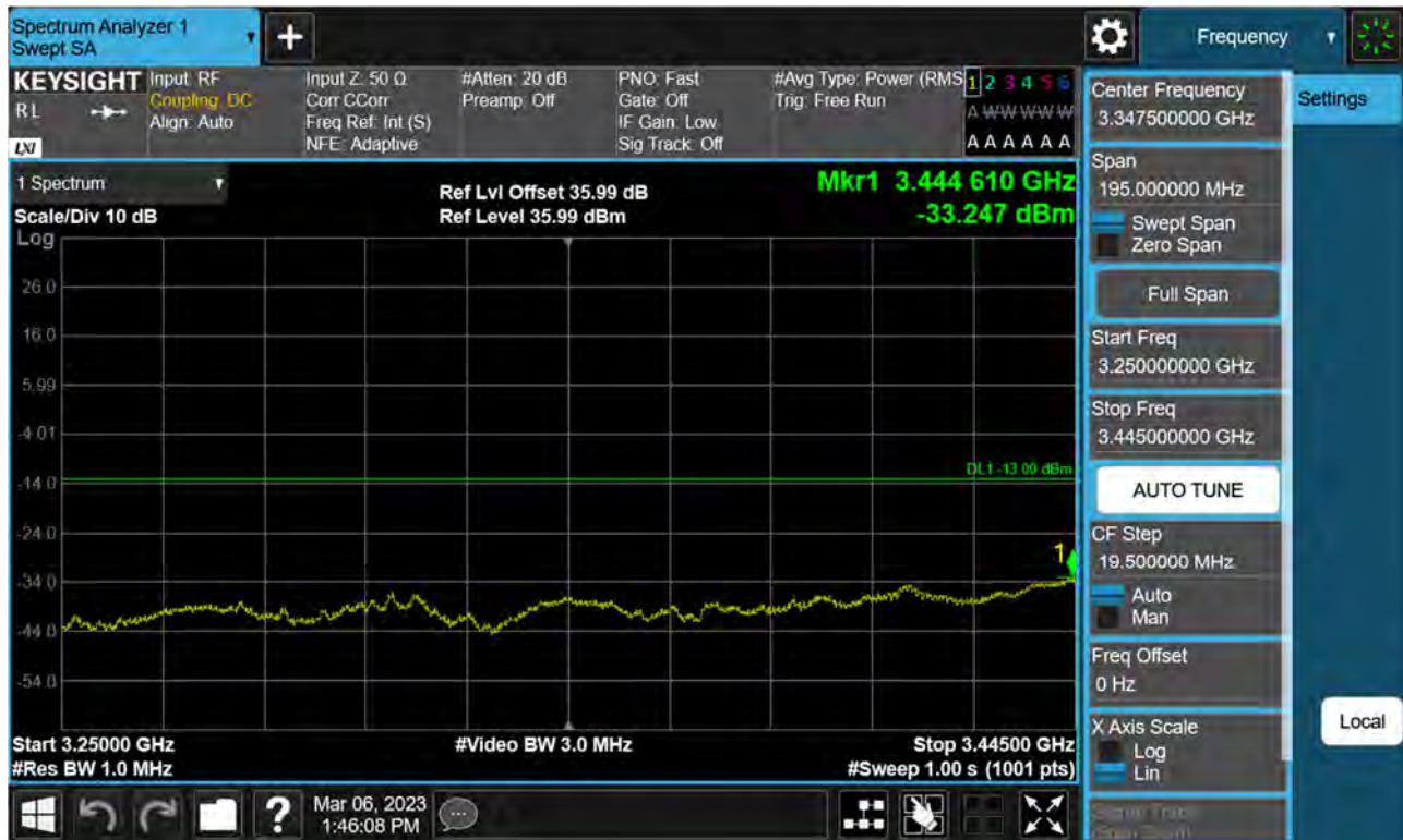
Sub6 n77(78). Low Band Edge Plot (80 M BW Ch.632668 BPSK FullIRB)(3)
