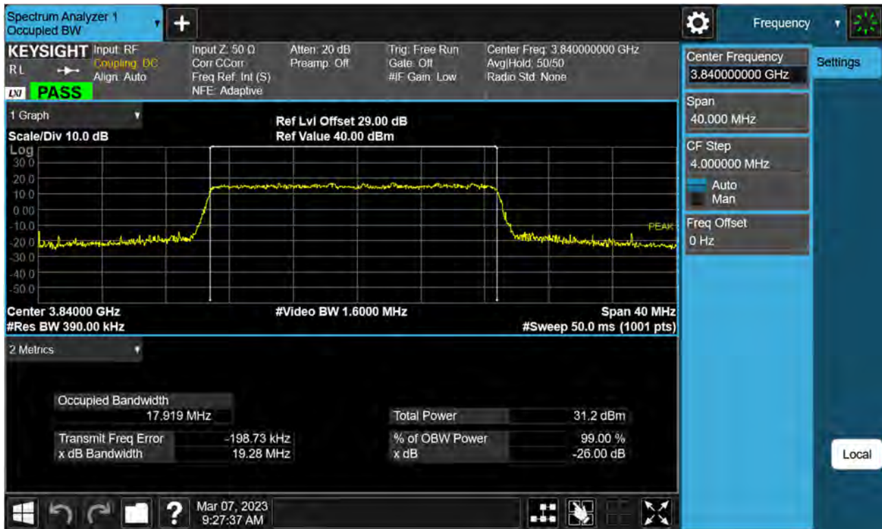
Sub6 n77(78). Occupied Bandwidth Plot (20 M BW Ch.656000 QPSK)
