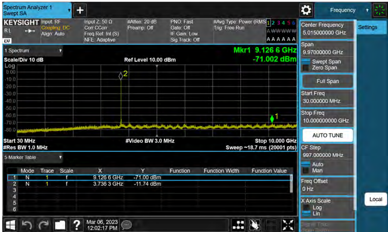
Sub6 n77(78). Conducted Spurious Plot_1 (633334ch_30 MHz_BPSK)
