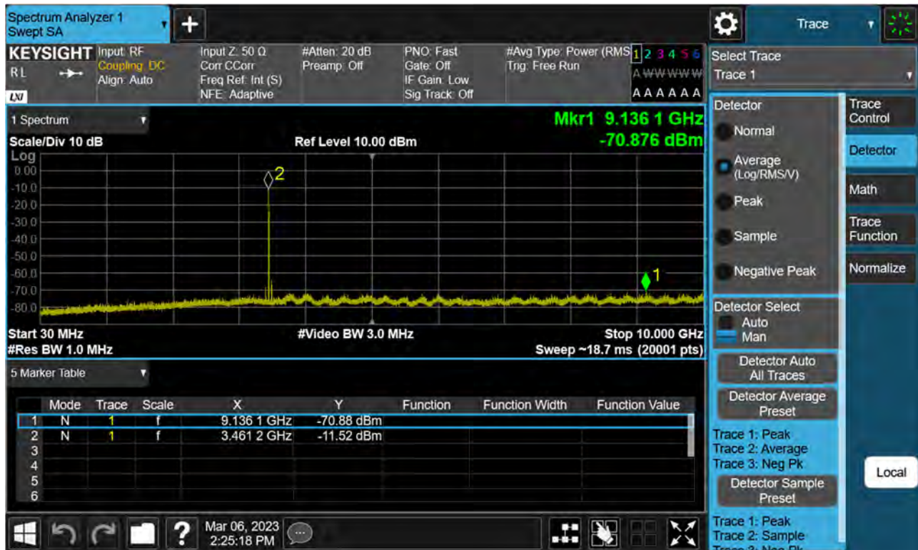
Sub6 n77(78). Conducted Spurious Plot_1 (633666ch_90 MHz_BPSK)
