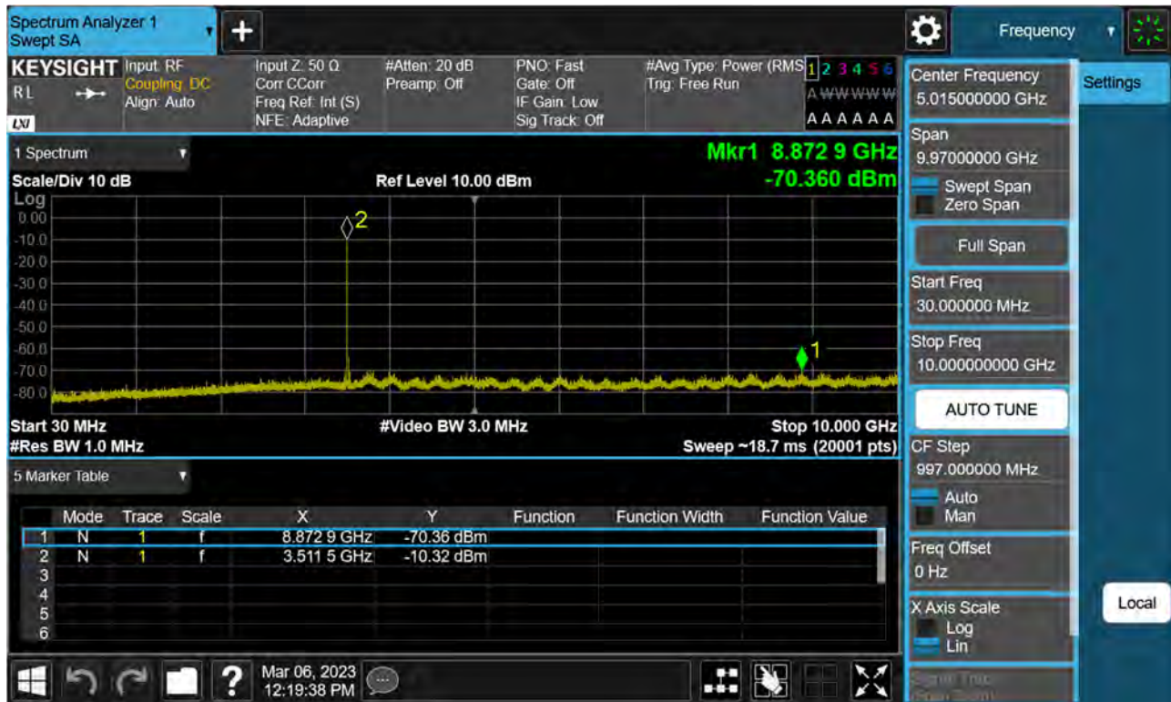
Sub6 n77(78). Conducted Spurious Plot_1 (635332ch_40 MHz_BPSK)
