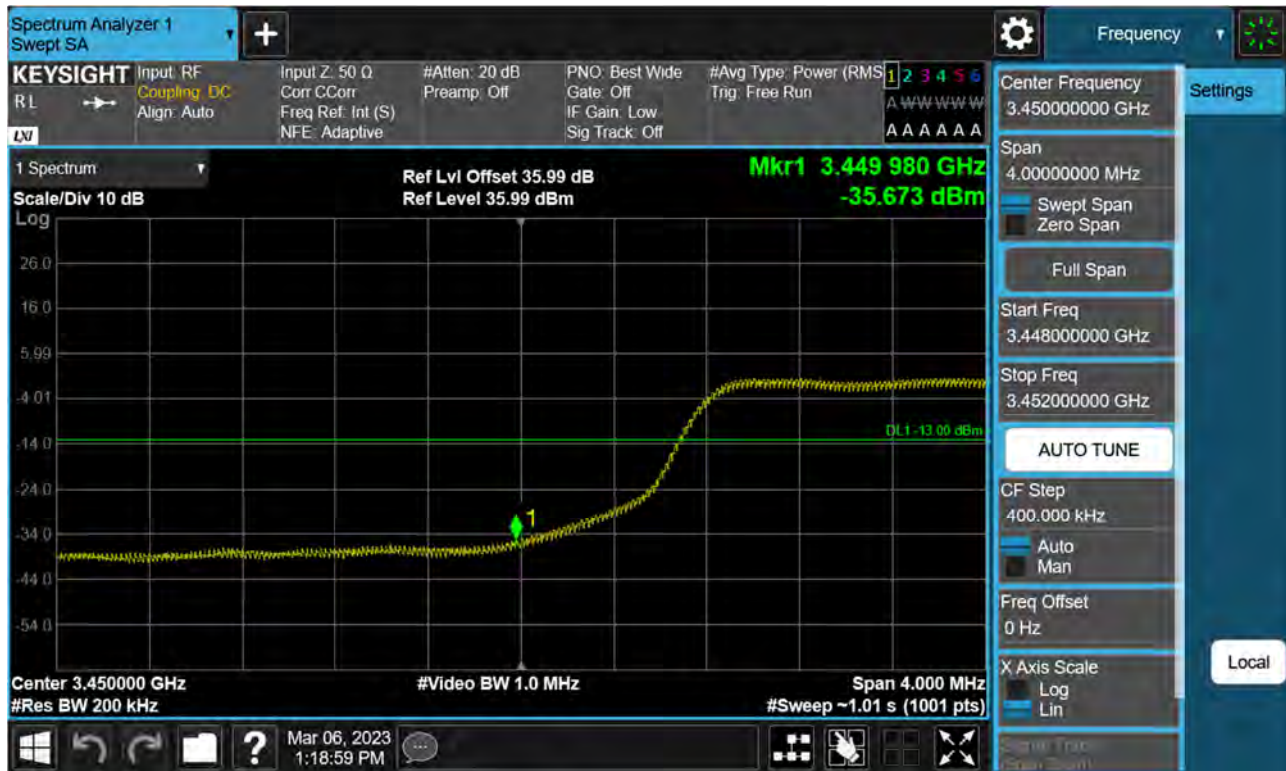
Sub6 n77(78). Low Band Edge Plot (60 M BW Ch.632000 BPSK FullRB)(1)
