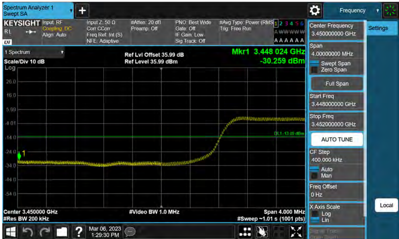
Sub6 n77(78). Low Band Edge Plot (70 M BW Ch.632334 BPSK FullRB)(1)
