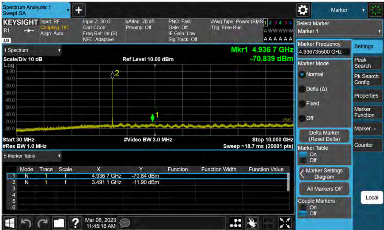
Sub6 n77(78). Conducted Spurious Plot_1 (633334ch_20 MHz_BPSK)
