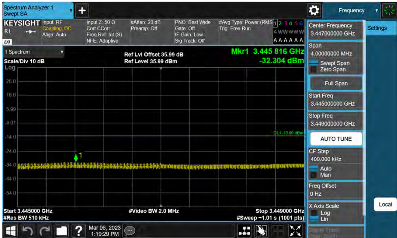
Sub6 n77(78). Low Band Edge Plot (60 M BW Ch.632000 BPSK FullRB)(2)
