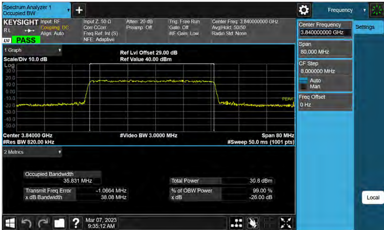
Sub6 n77(78). Occupied Bandwidth Plot (40 M BW Ch.656000 16QAM)
