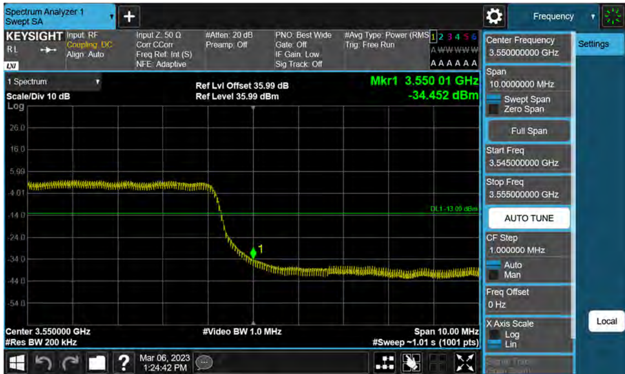
Sub6 n77(78). High Band Edge Plot (60 M BW Ch.634666 BPSK FullRB)(1)
