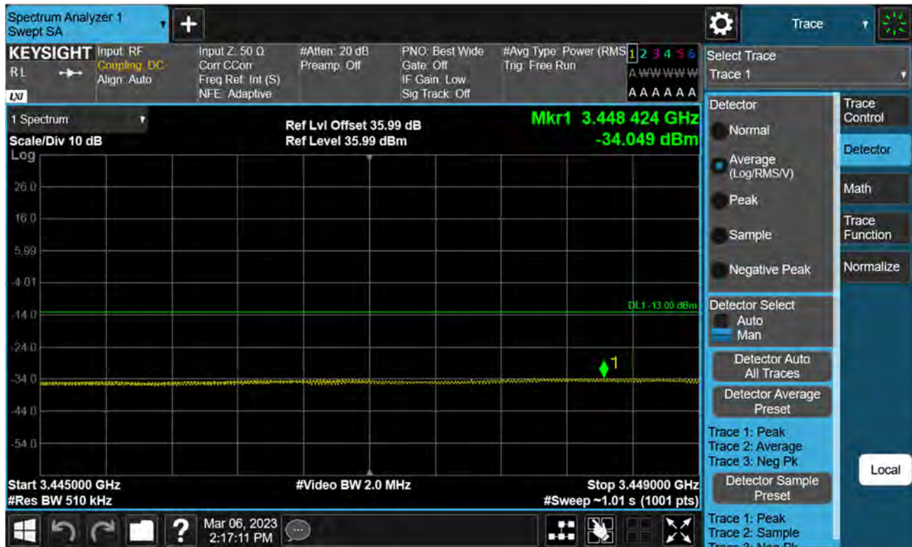
Sub6 n77(78). Low Band Edge Plot (90 M BW Ch.633000 BPSK FullIRB)(2)
