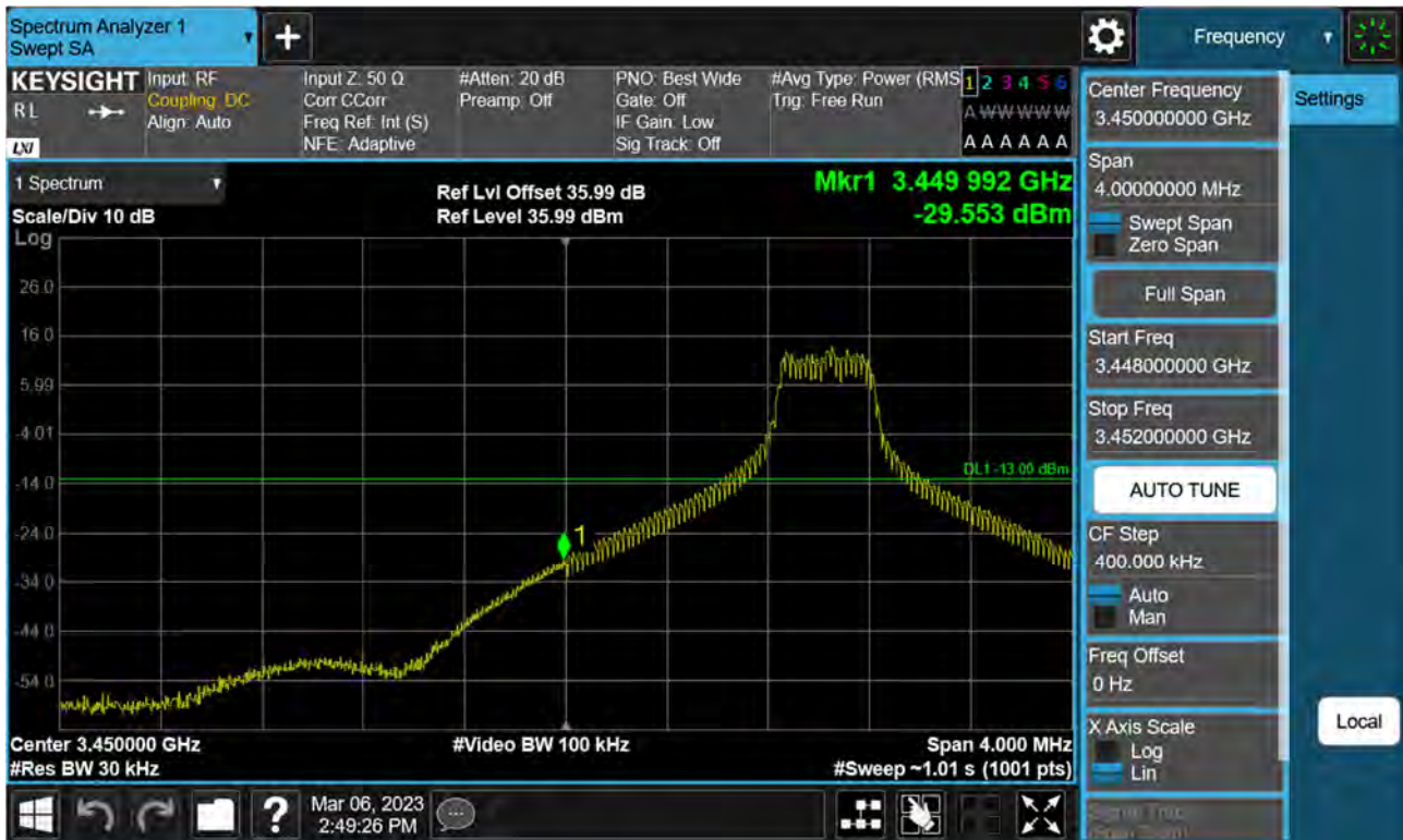
Sub6 n77(78). Low Band Edge Plot (100 M BW Ch.633334 BPSK 1RB)(1)
