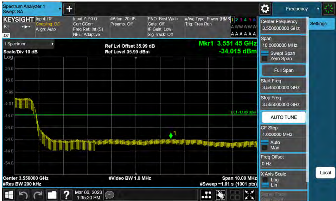
Sub6 n77(78). High Band Edge Plot (70 M BW Ch.634332 BPSK FullRB)(1)
