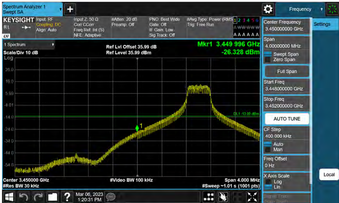
Sub6 n77(78). Low Band Edge Plot (60 M BW Ch.632000 BPSK 1RB)(1)
