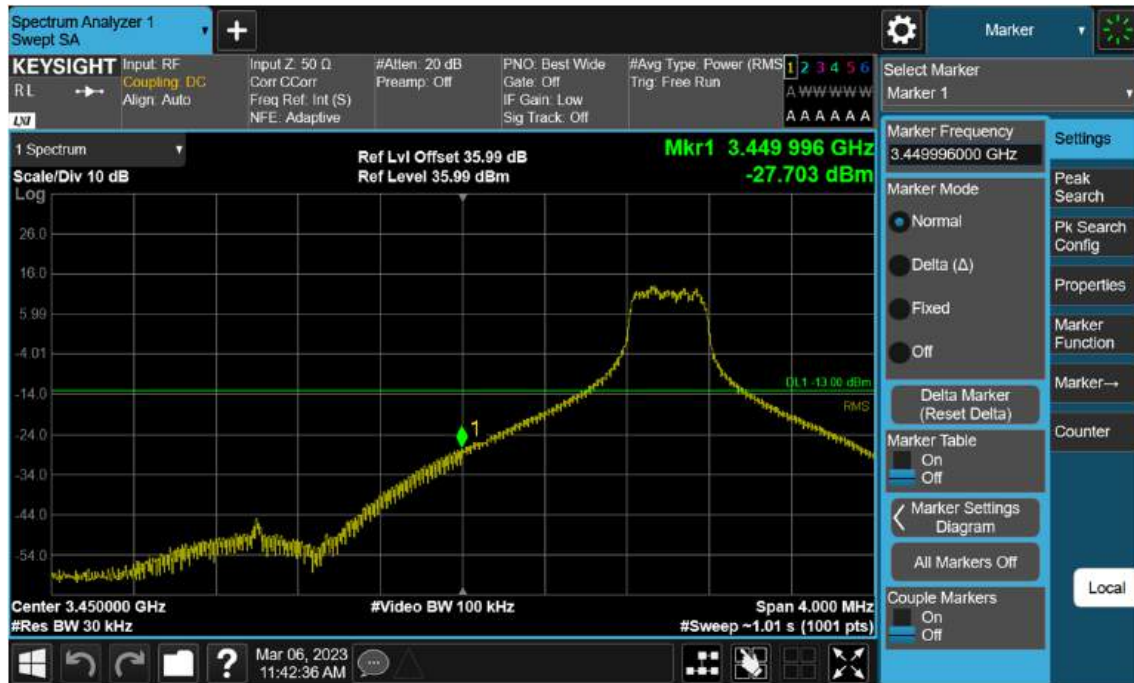
Sub6 n77(78). Low Band Edge Plot (20 M BW Ch.630668 BPSK 1RB)(1)
