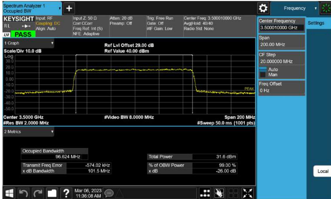
Sub6 n77(78). Occupied Bandwidth Plot (100 M BW Ch.633334 64 QAM )
