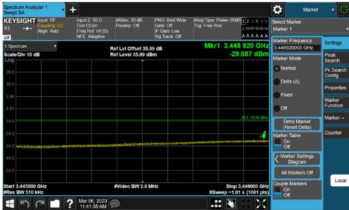
Sub6 n77(78). Low Band Edge Plot (20 M BW Ch.630668 BPSK FullRB)(2)
