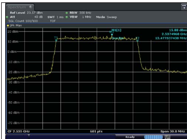
15 MHz QPSK Middle Channel - Full RB
