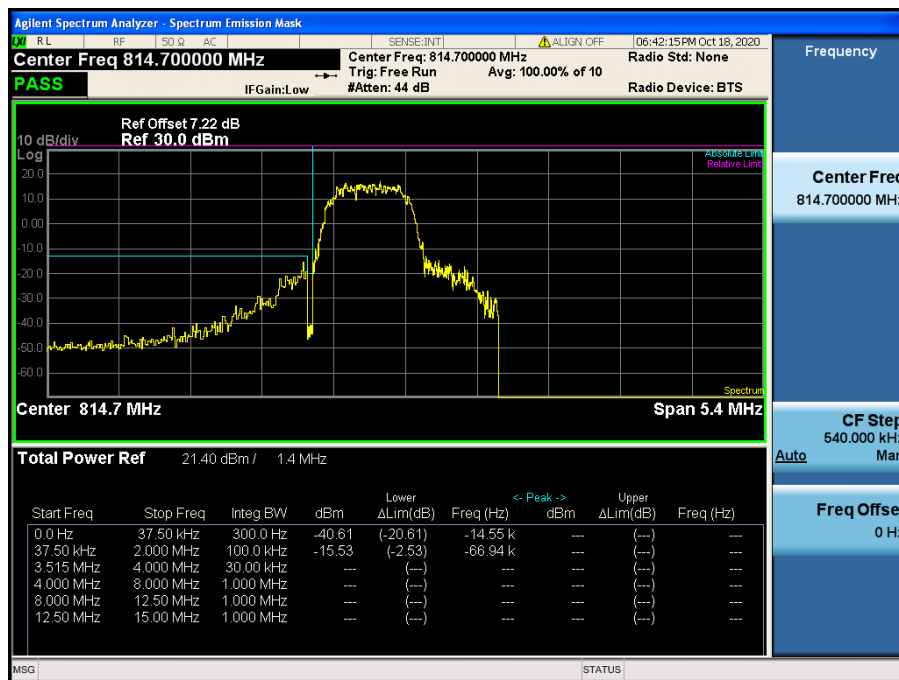
LTE Band 26 / 1.4 MHz / 16QAM - RB Size/Offset (3/0)
