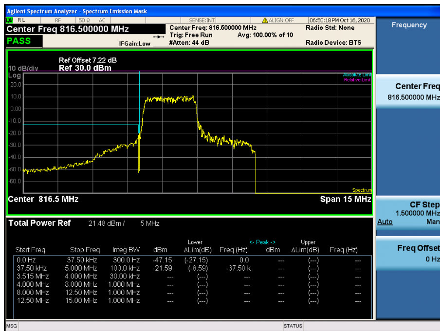
LTE Band 26 / 5 MHz / QPSK - RB Size/Offset (12/0)
