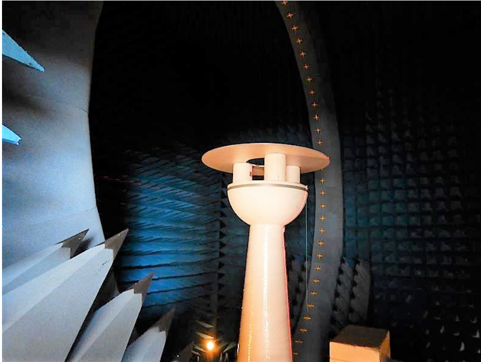
1m groundplane inside Satimo SG64 anechoic chamber
