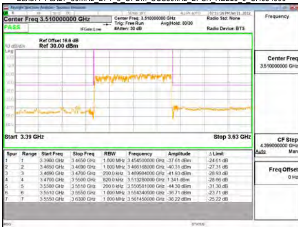
Band77-Part27 80MHz DFT s OFDM SCS30kHz BPSK RB216 0 CH634000
