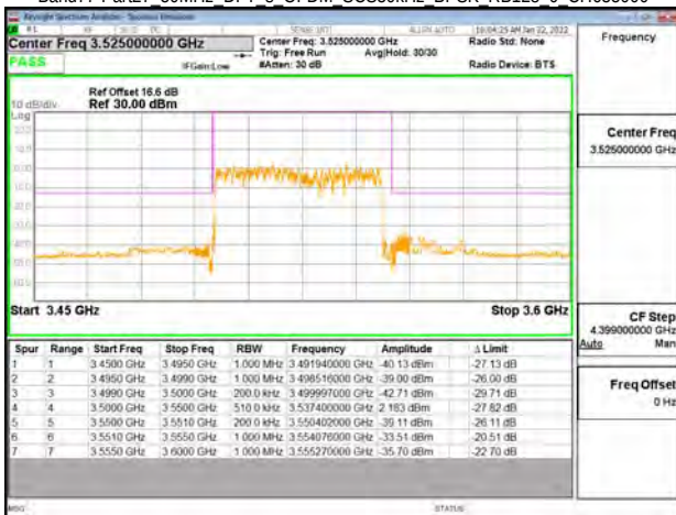
Band77-Part27 50MHz DFT s OFDM SCS30kHz BPSK RB128 0 CH635000
