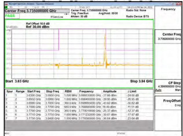
Band77-Part27 70MHz DFT s OFDM SCS30kHz BPSK RB1 188 CH656000
