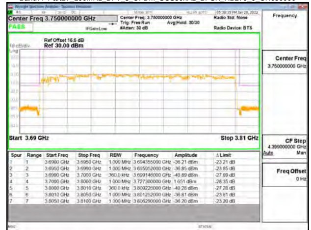
Band77-Part27 100MHz DFT s OFDM SCS30kHz BPSK RB270 0 CH656000
