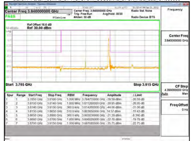
Band77-Part27 50MHz DFT s OFDM SCS30kHz BPSK RB1 132 CH636666
