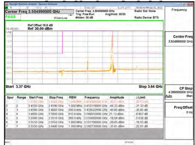
Band77-Part27 90MHz DFT s OFDM SCS30kHz BPSK RB1 244 CH649668
