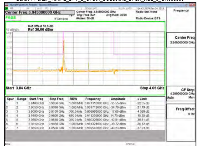
Band77-Part27 70MHz DFT s OFDM SCS30kHz BPSK RB1 0 CH663000
