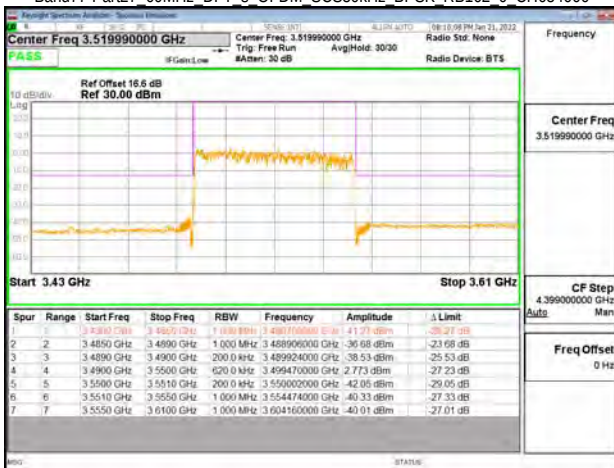
Band77-Part27 60MHz DFT s OFDM SCS30kHz BPSK RB162 0 CH634666
