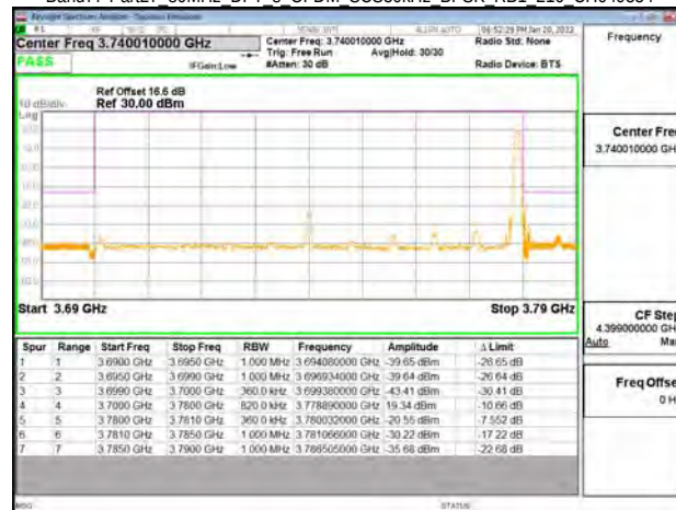
Band77-Part27 80MHz DFT s OFDM SCS30kHz BPSK RB1 216 CH656000
