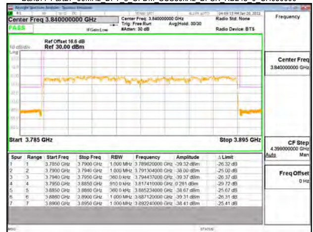
Band77-Part27 90MHz DFT s OFDM SCS30kHz BPSK RB243 0 CH656000
