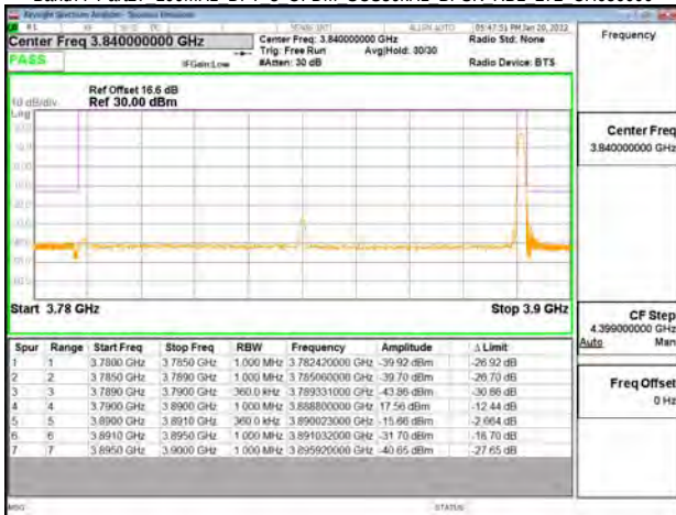
Band77-Part27 100MHz DFT s OFDM SCS30kHz BPSK RB1 272 CH620000
