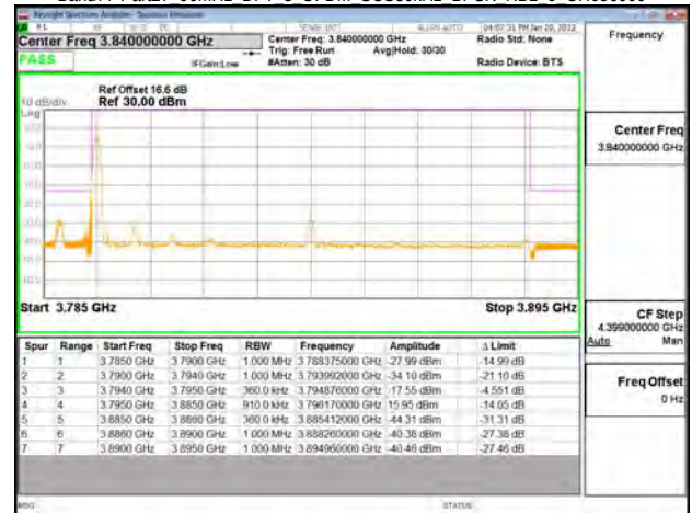
Band77-Part27 90MHz DFT s OFDM SCS30kHz BPSK RB1 0 CH662332
