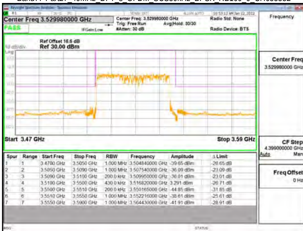
Band77-Part27 40MHz DFT s OFDM SCS30kHz BPSK RB100 0 CH635332
