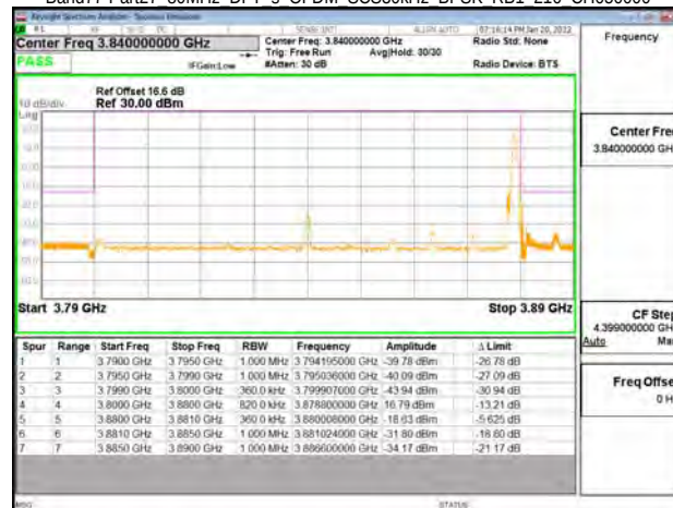
Band77-Part27 80MHz DFT s OFDM SCS30kHz BPSK RB1 216 CH626666
