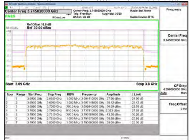
Band77-Part27 90MHz DFT s OFDM SCS30kHz BPSK RB243 0 CH656000
