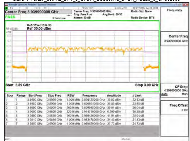
Band77-Part27 80MHz DFT s OFDM SCS30kHz BPSK RB216 0 CH626666
