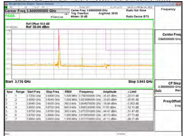
Band77-Part27 70MHz DFT s OFDM SCS30kHz BPSK RB1 0 CH663000
