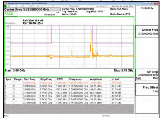
Band77-Part27 40MHz DFT s OFDM SCS30kHz BPSK RB1_105 CH656000
