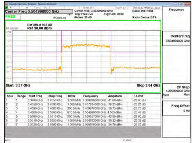
Band77-Part27 90MHz DFT s OFDM SCS30kHz BPSK RB243 0 CH649668
