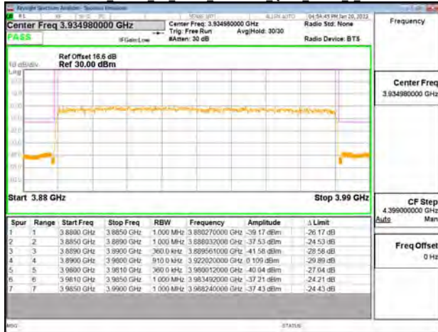
Band77-Part27 100MHz DFT s OFDM SCS30kHz BPSK RB1 0 CH633334
