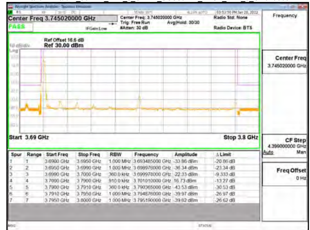
Band77-Part27 90MHz DFT s OFDM SCS30kHz BPSK RB1 0 CH656000
