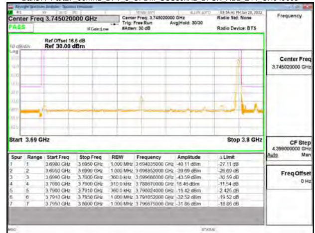
Band77-Part27 90MHz DFT s OFDM SCS30kHz BPSK RB1 244 CH656000
