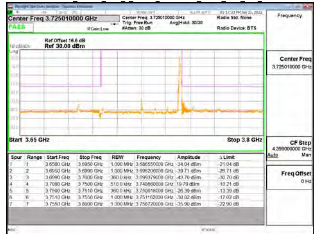
Band77-Part27 50MHz DFT s OFDM SCS30kHz BPSK RB1 132 CH656000
