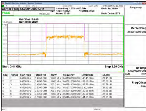
Band77-Part27 60MHz DFT s OFDM SCS30kHz BPSK RB162 0 CH634666
