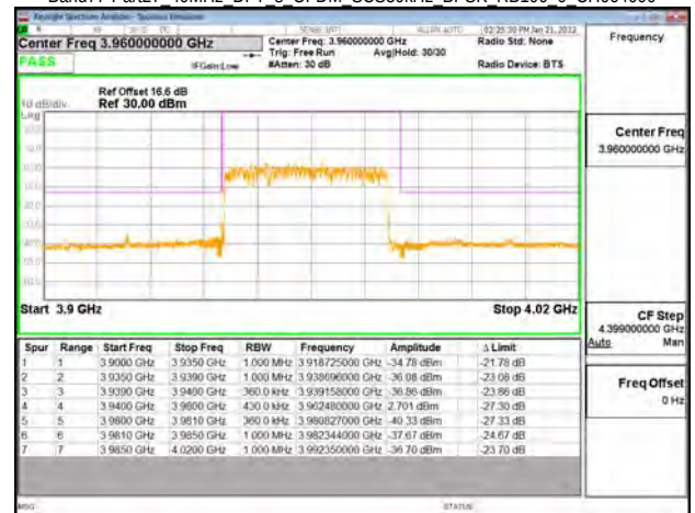
Band77-Part27 40MHz DFT s OFDM SCS30kHz BPSK RB100 0 CH664000
