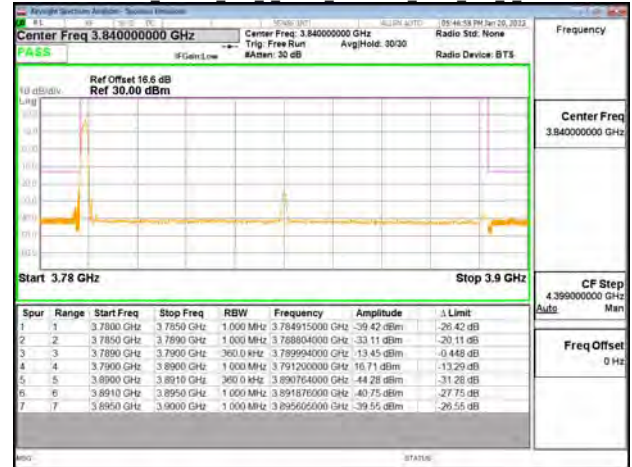
Band77-Part27 100MHz DFT s OFDM SCS30kHz BPSK RB1 0 CH662000
