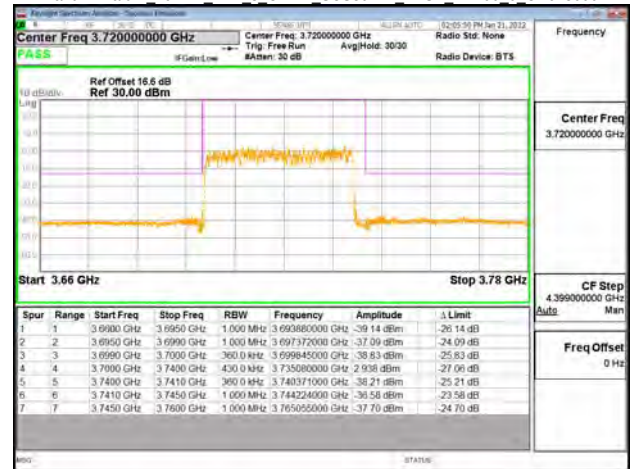
Band77-Part27 40MHz DFT s OFDM SCS30kHz BPSK RB100 0 CH656000
