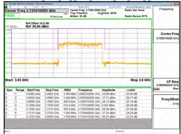
Band77-Part27 50MHz DFT s OFDM SCS30kHz BPSK RB128 0 CH656000
