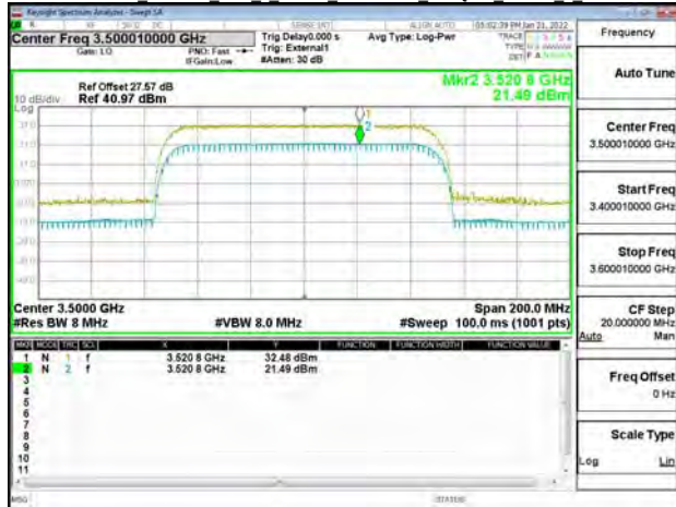
Band77-Part27 20MHz DFT s OFDM SCS30kHz 256QAM RB50 0 CH647334
