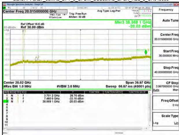
Band77-Part27 60MHz DFT s OFDM SCS30kHz BPSK RB1 1 CH656000
