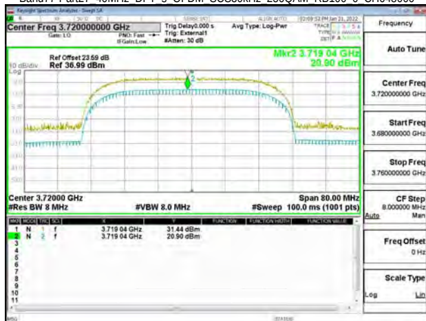
Band77-Part27 40MHz DFT s OFDM SCS30kHz 256QAM RB100 0 CH656000
