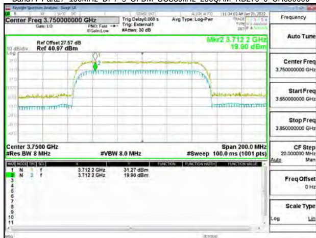
Band77-Part27 100MHz DFT s OFDM SCS30kHz 256QAM RB270 0 CH650000
