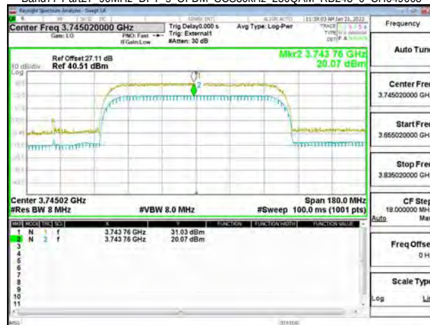
Band77-Part27 90MHz DFT s OFDM SCS30kHz 256QAM RB243 0 CH656000
