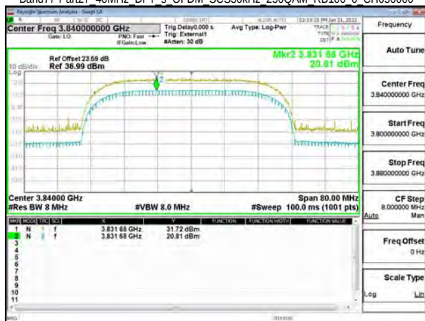
Band77-Part27 40MHz DFT s OFDM SCS30kHz 256QAM RB100 0 CH656000
