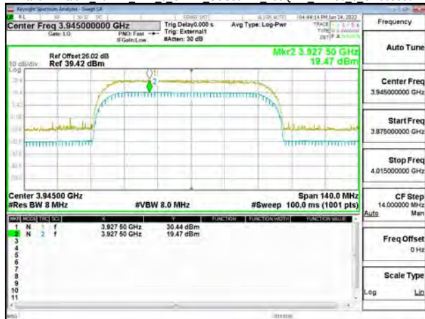
Band77-Part27 80MHz DFT s OFDM SCS30kHz 256QAM RB216 0 CH649334
