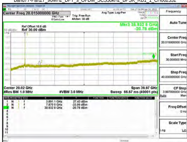
Band77-Part27 90MHz DFT s OFDM SCS30kHz BPSK RB1 1 CH662332
