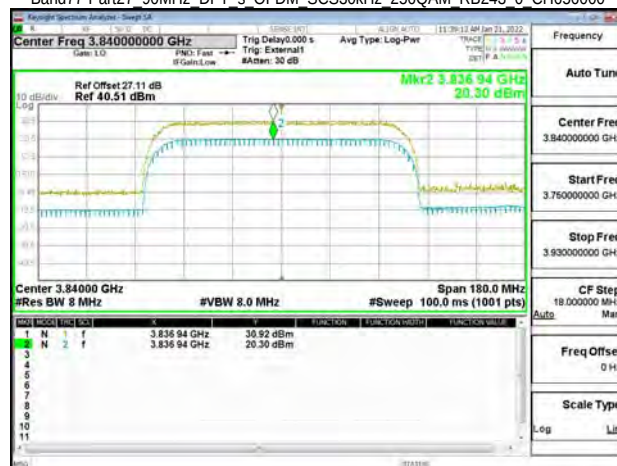
Band77-Part27 90MHz DFT s OFDM SCS30kHz 256QAM RB243 0 CH656000
