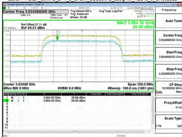
Band77-Part27 100MHz DFT s OFDM SCS30kHz 256QAM RB270 0 CH650000
