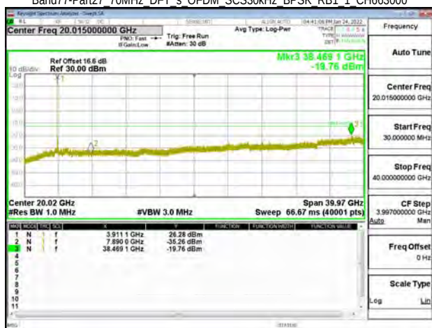
Band77-Part27 70MHz DFT s OFDM SCS30kHz BPSK RB1 1 CH663000
