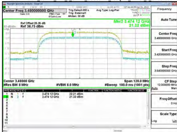
Band77-Part27 60MHz DFT s OFDM SCS30kHz 256QAM RB162 0 CH633334
