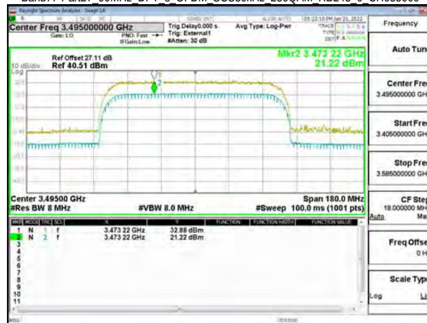
Band77-Part27 90MHz DFT s OFDM SCS30kHz 256QAM RB243 0 CH633334
