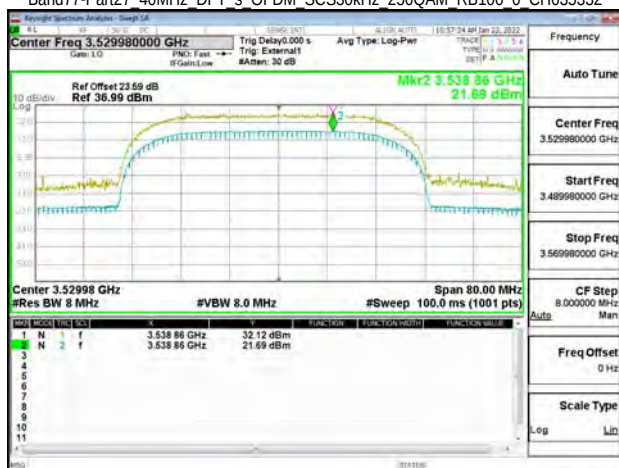
Band77-Part27 40MHz DFT s OFDM SCS30kHz 256QAM RB100 0 CH635332
