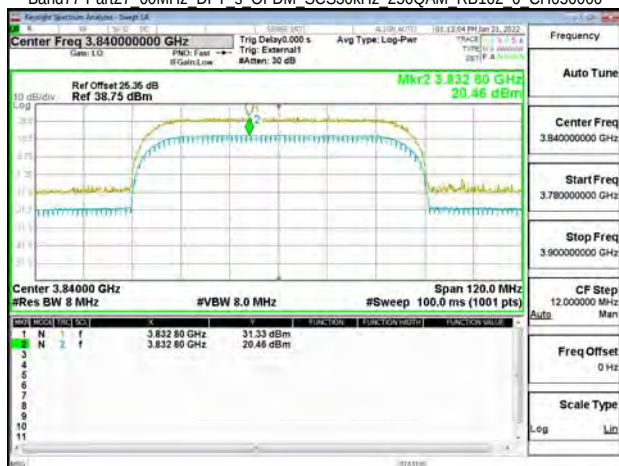
Band77-Part27 60MHz DFT s OFDM SCS30kHz 256QAM RB162 0 CH656000
