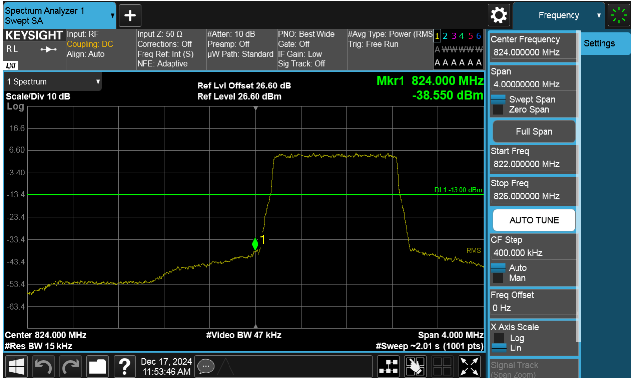
BAND 26(5). Lower Band Edge Plot (1.4 M BW Ch.26797 QPSK_RB6_Offset 0)
