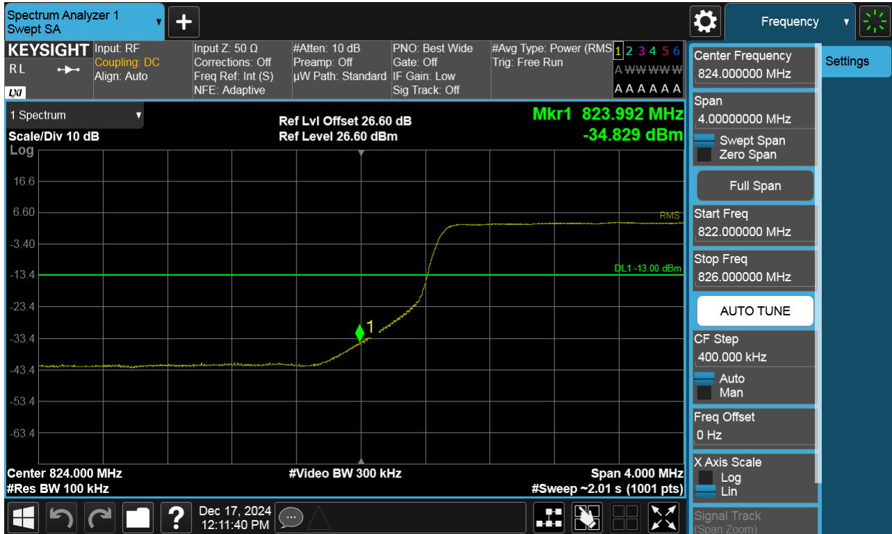
BAND 26(5). Lower Band Edge Plot (10 M BW Ch.26840 QPSK_RB50_Offset 0)
