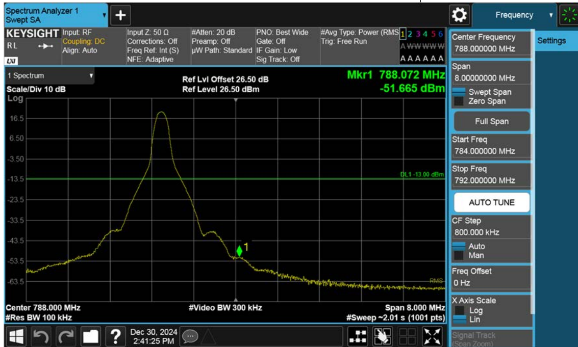
Sub6 n13_10 M_Band Edge_High_BPSK_1RB
