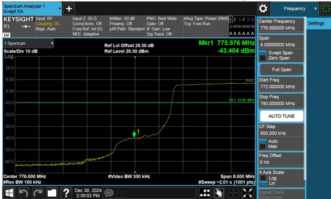
Sub6 n13_10 M_Band Edge_Low_BPSK_FullIRB
