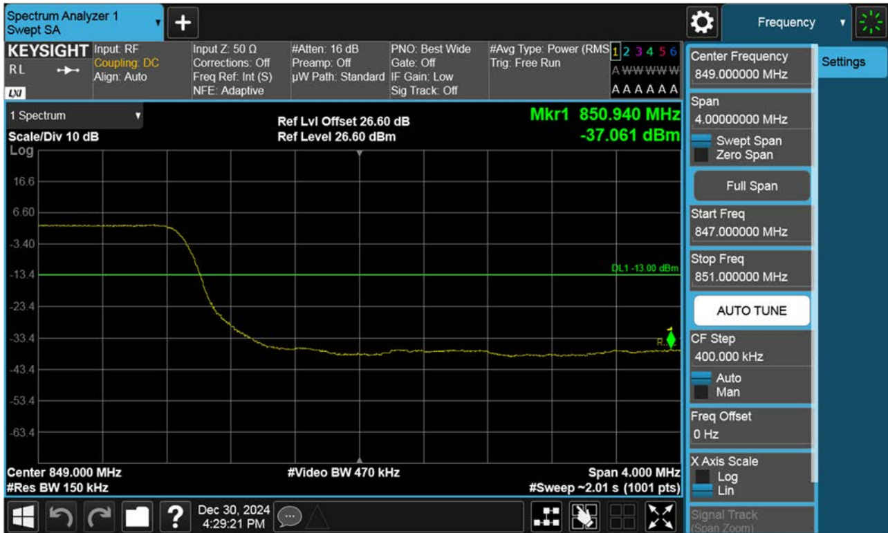
Upper Band Edge Plot (15 M BW Ch.168300 BPSK_RB 75_Offset 0)
