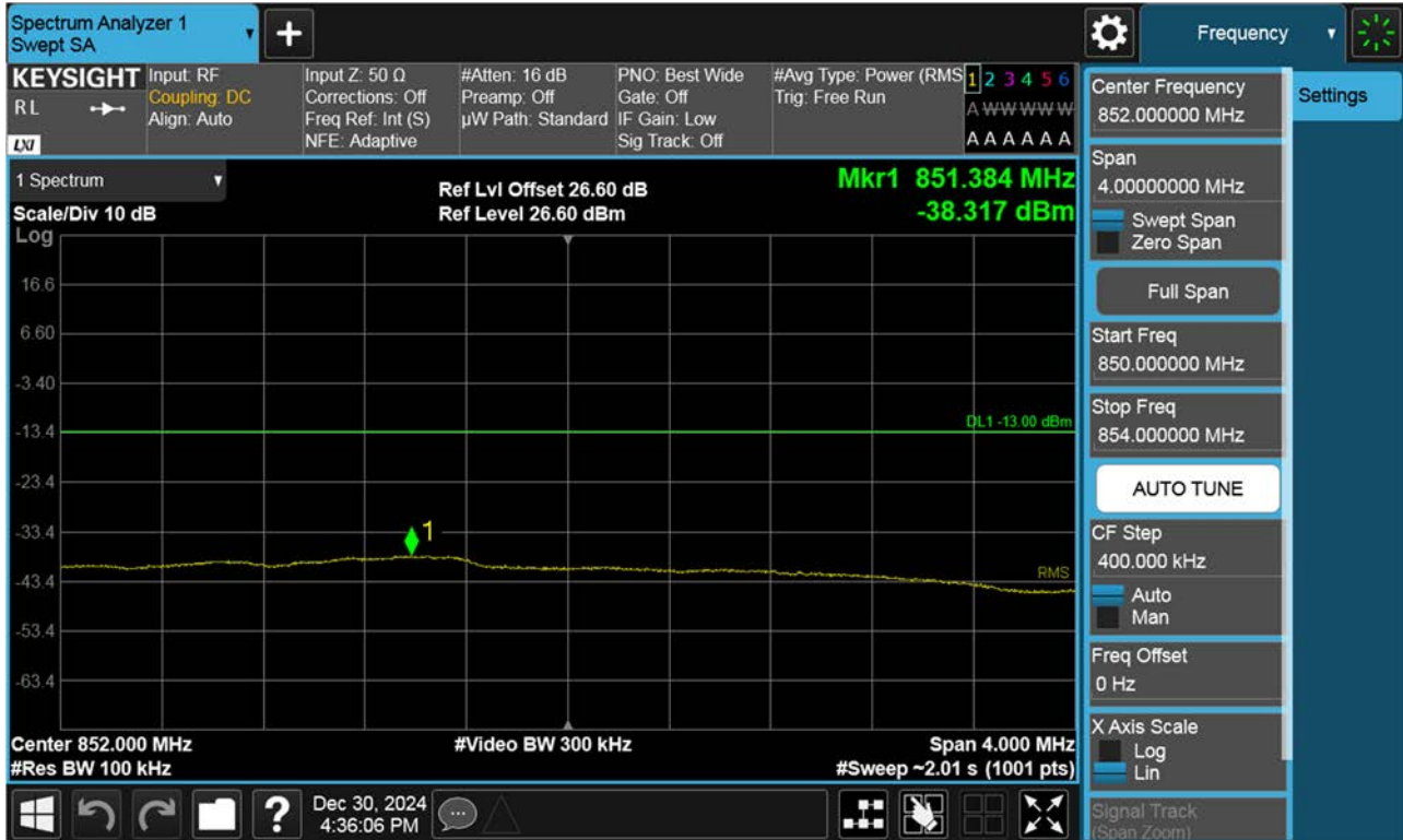
Upper Extended Band Edge Plot (20 M BW Ch.167800 BPSK_RB 100_0)
