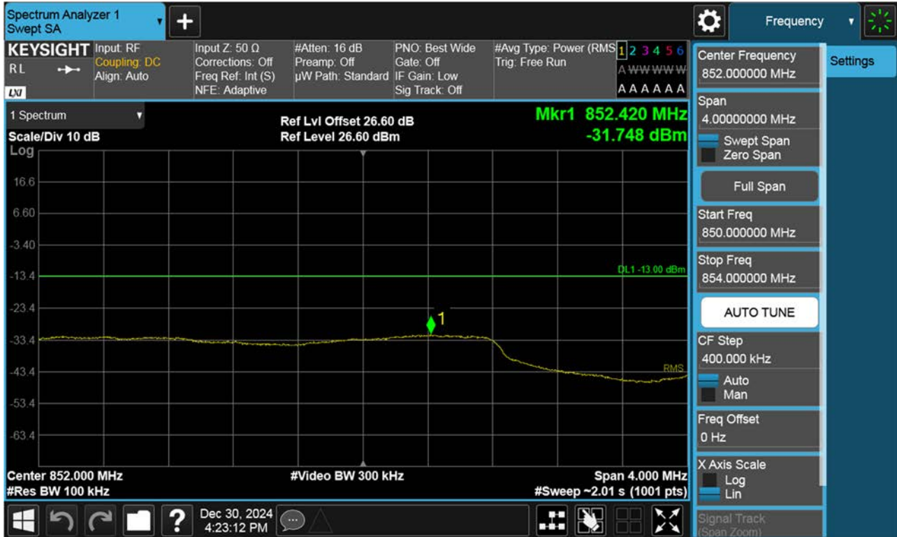
Upper Extended Band Edge Plot (10 M BW Ch.168800 BPSK_RB 50_0)
