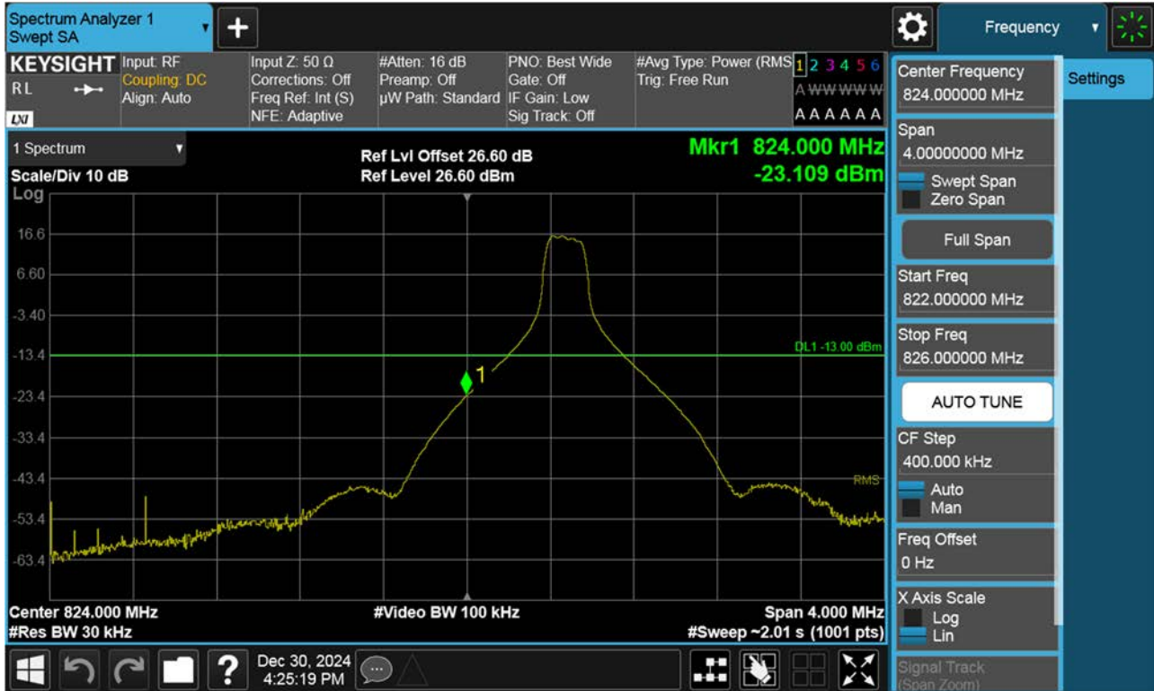
Lower Band Edge Plot (15 M BW Ch.166300 BPSK_RB 1_Offset 0)
