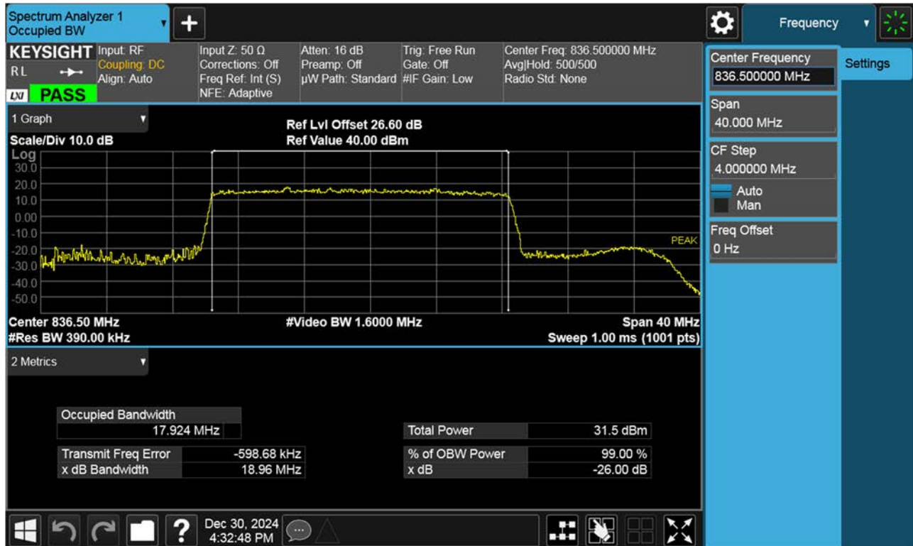
Occupied Bandwidth Plot (20 M BW Ch.167300 BPSK RB 100_0)
