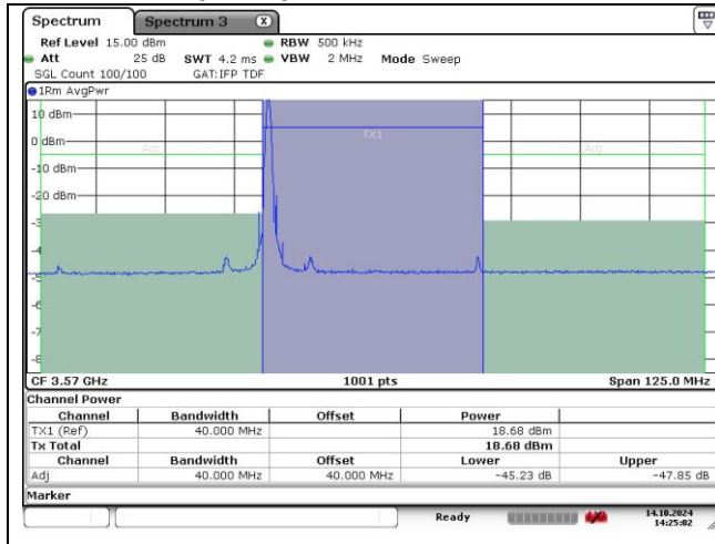
DFT-S-OFDM BPSK - Low Channel - 1 RB
