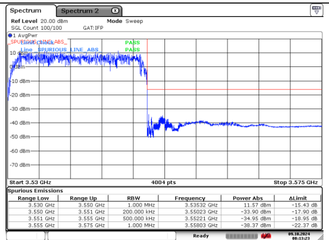
DFT-S-OFDM QPSK - High Channel - Full RB
