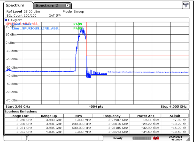
CP-OFDM 16QAM - High Channel - 1 RB
