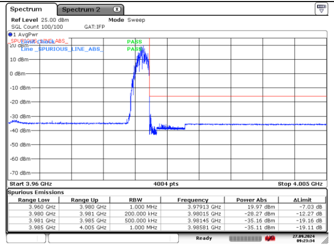
CP-OFDM 16QAM - High Channel - 1 RB
