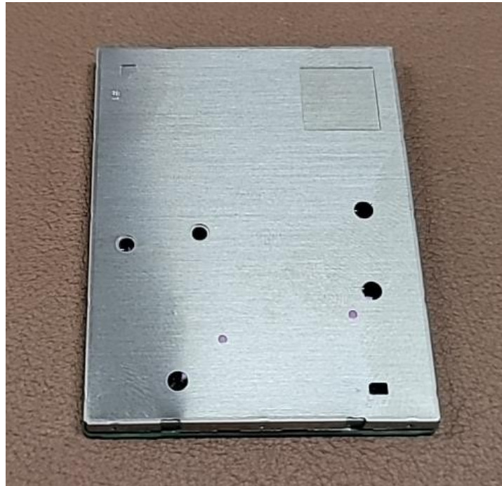
Installation of Shield-can cover
