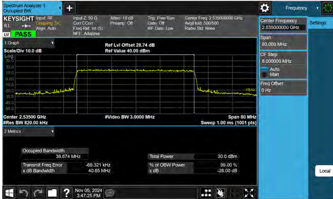
Sub6 n7. Occupied Bandwidth Plot (40 M BW Ch.507000 64QAM)
