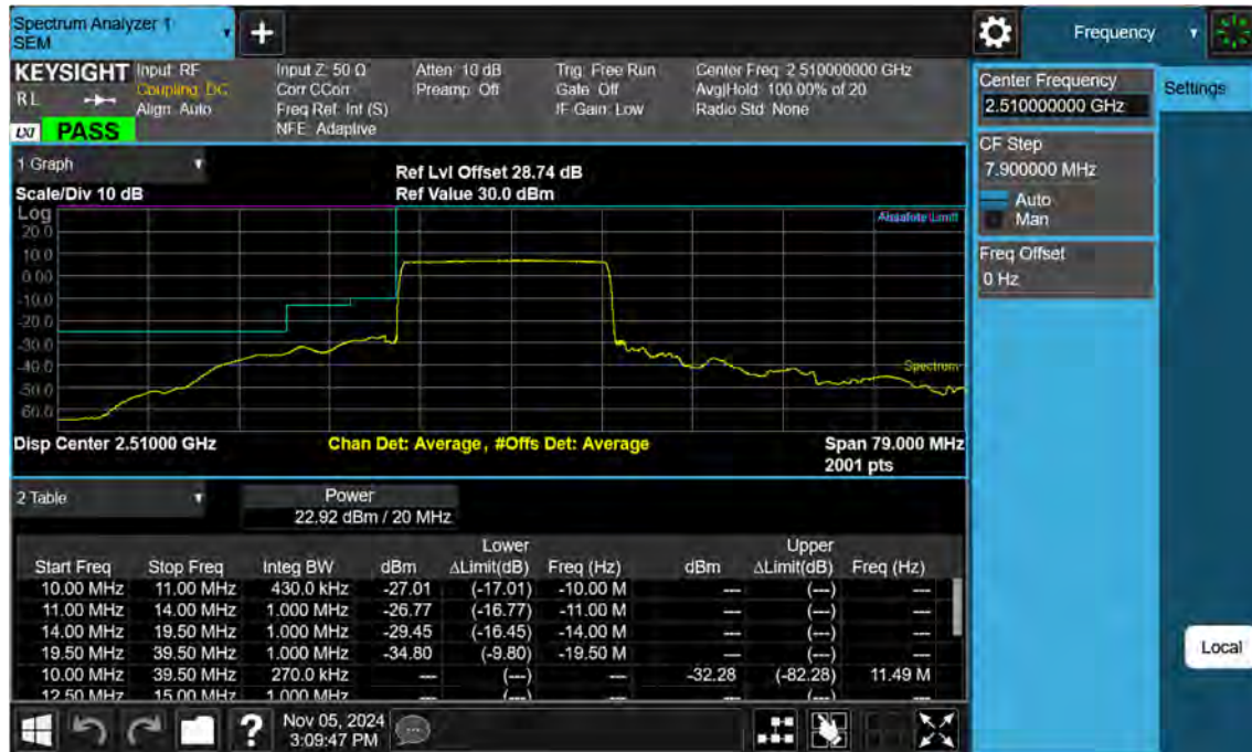
Sub6 n7. Low Channel Edge Plot (20 MHz Ch.502000 BPSK)-1
