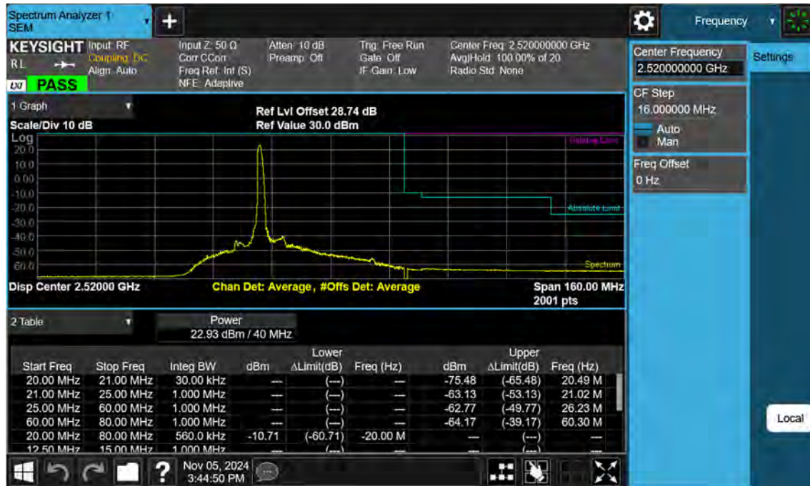
Sub6 n7. Low Channel Edge Plot (40 MHz Ch.504000 BPSK_RB1)-2
