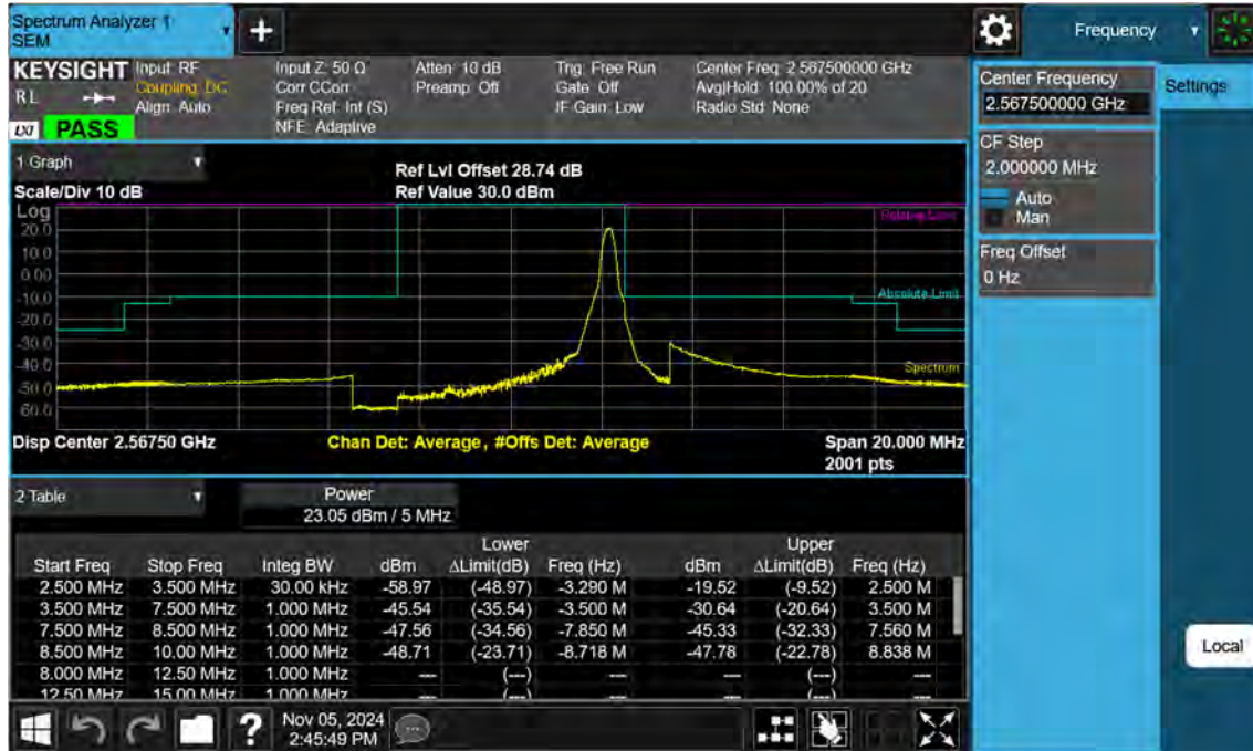
Sub6 n7. High Channel Edge Plot (5 MHz Ch.513500 BPSK RB 1)
