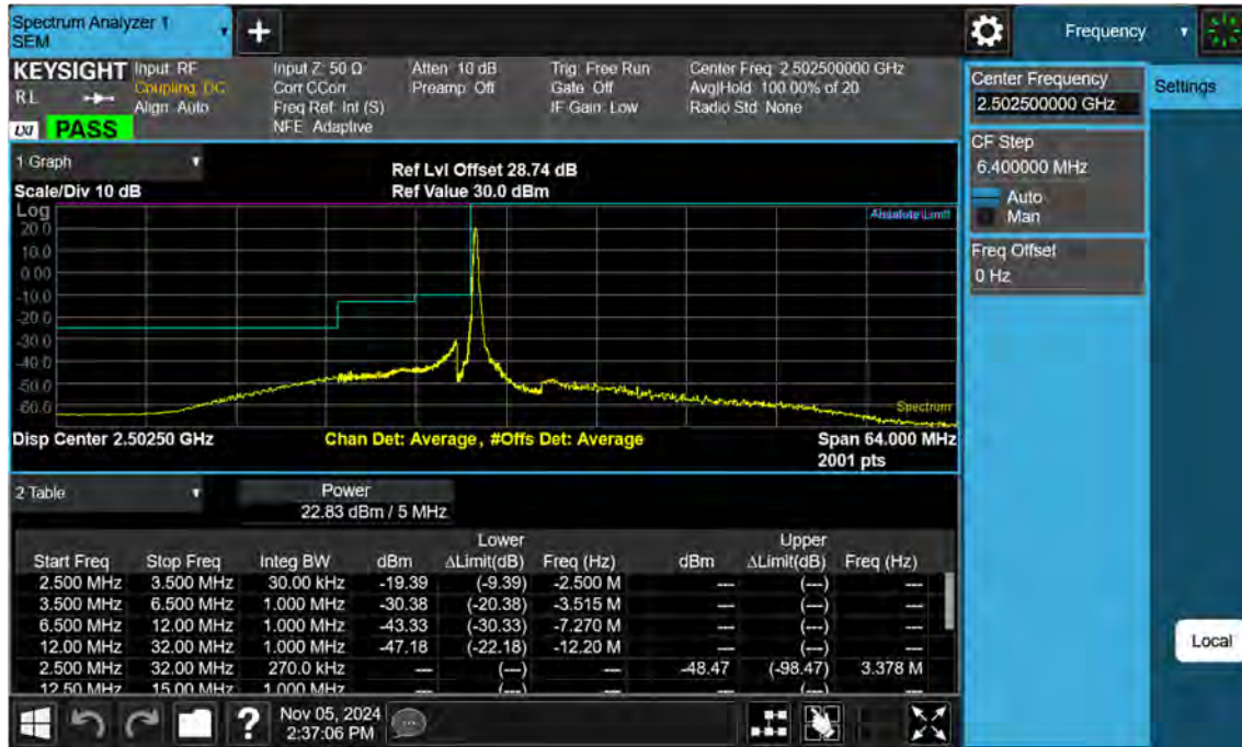
Sub6 n7. Low Channel Edge Plot (5 MHz Ch.500500 BPSK RB 1)-1
