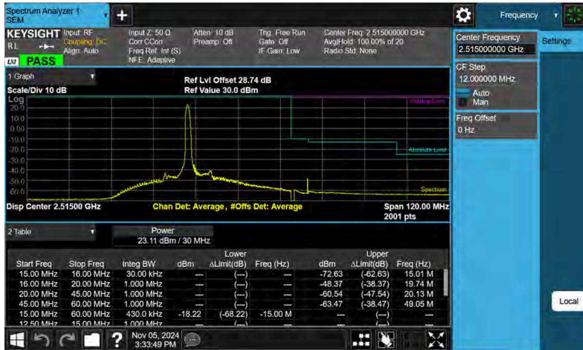
Sub6 n7. Low Channel Edge Plot (30 MHz Ch.503000 BPSK_RB1)-2
