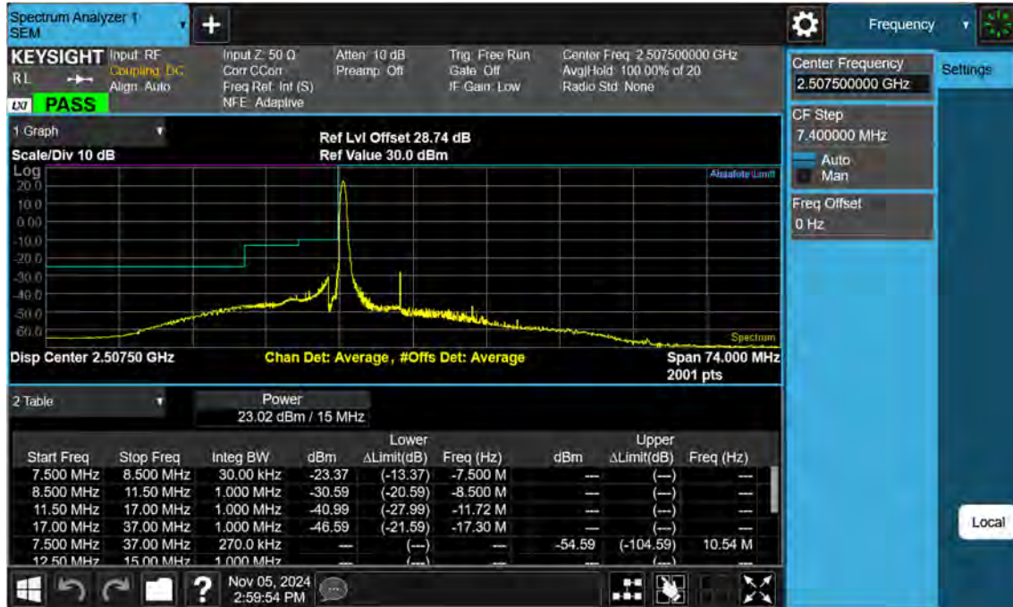
Sub6 n7. Low Channel Edge Plot (15 MHz Ch.501500 BPSK RB 1)-1
