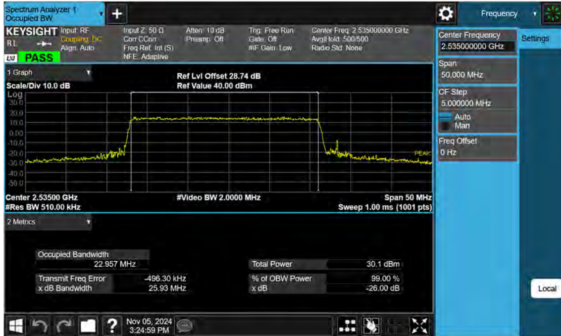
Sub6 n7. Occupied Bandwidth Plot (25 M BW Ch.507000 16QAM)
