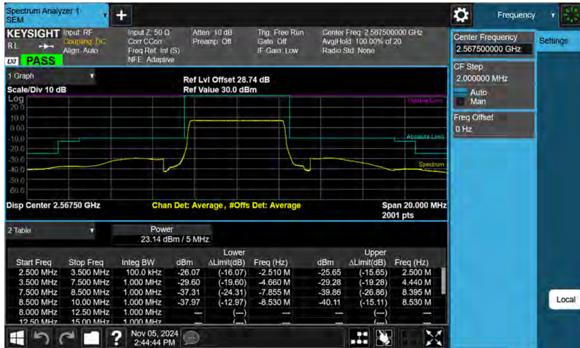
Sub6 n7. High Channel Edge Plot (5 MHz Ch.513500 BPSK)
