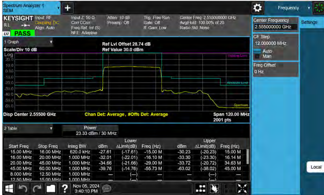
Sub6 n7. High Channel Edge Plot (30 MHz Ch.511000 BPSK)
