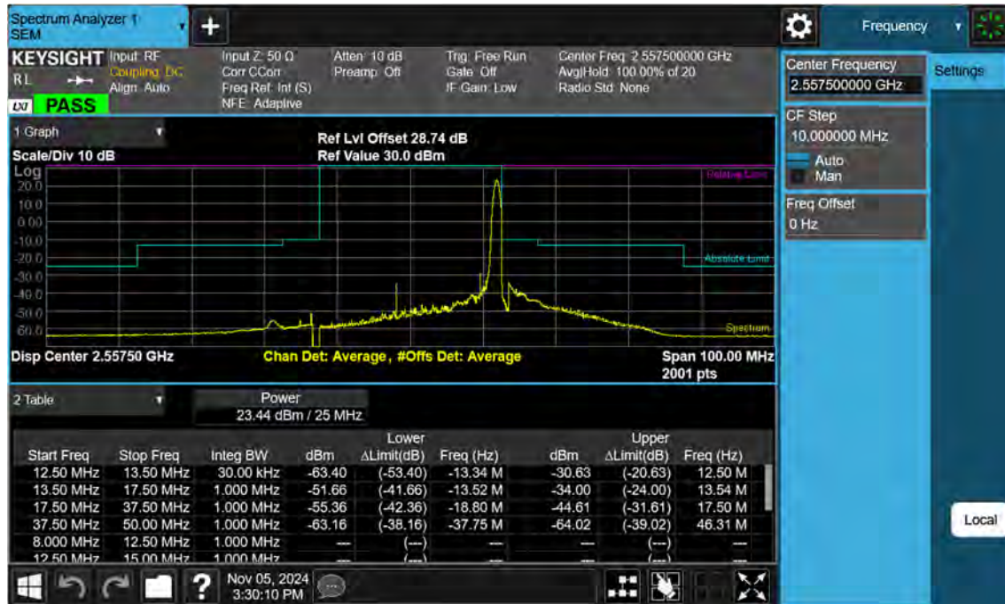
Sub6 n7. High Channel Edge Plot (25 MHz Ch.511500 BPSK RB 1)
