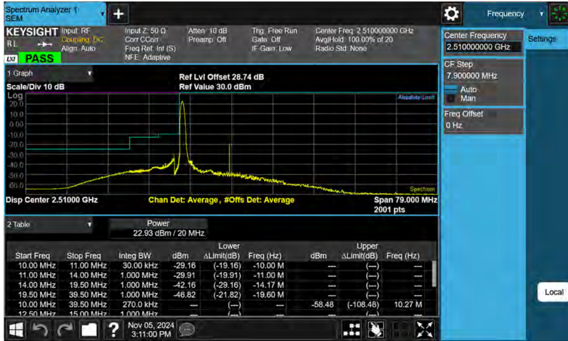
Sub6 n7. Low Channel Edge Plot (20 MHz Ch.502000 BPSK RB 1)-1
