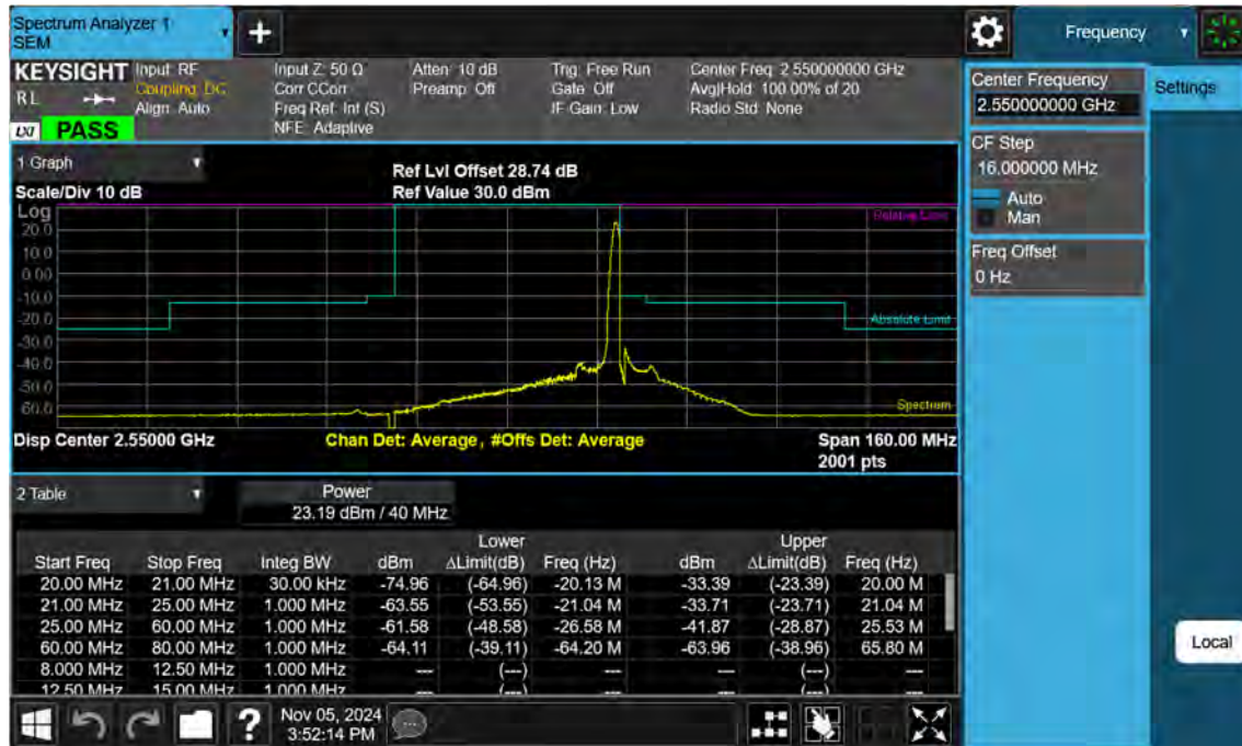
Sub6 n7. High Channel Edge Plot (40 MHz Ch.510000 BPSK RB 1)
