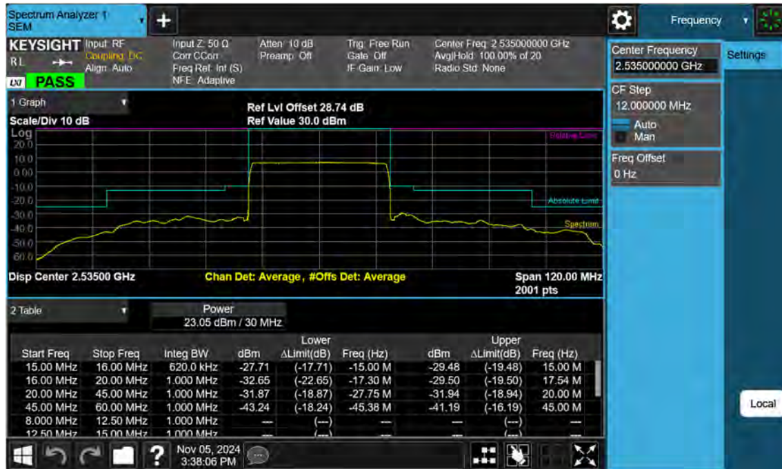
Sub6 n7. Mid Channel Edge Plot (30 MHz Ch.507000 BPSK)
