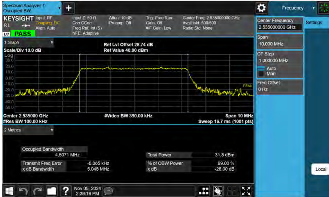
Sub6 n7. Occupied Bandwidth Plot (5 M BW Ch.507000 BPSK)
