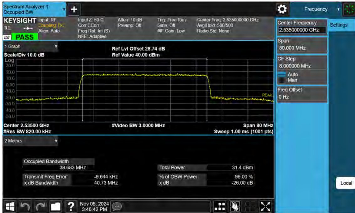
Sub6 n7. Occupied Bandwidth Plot (40 M BW Ch.507000 QPSK)
