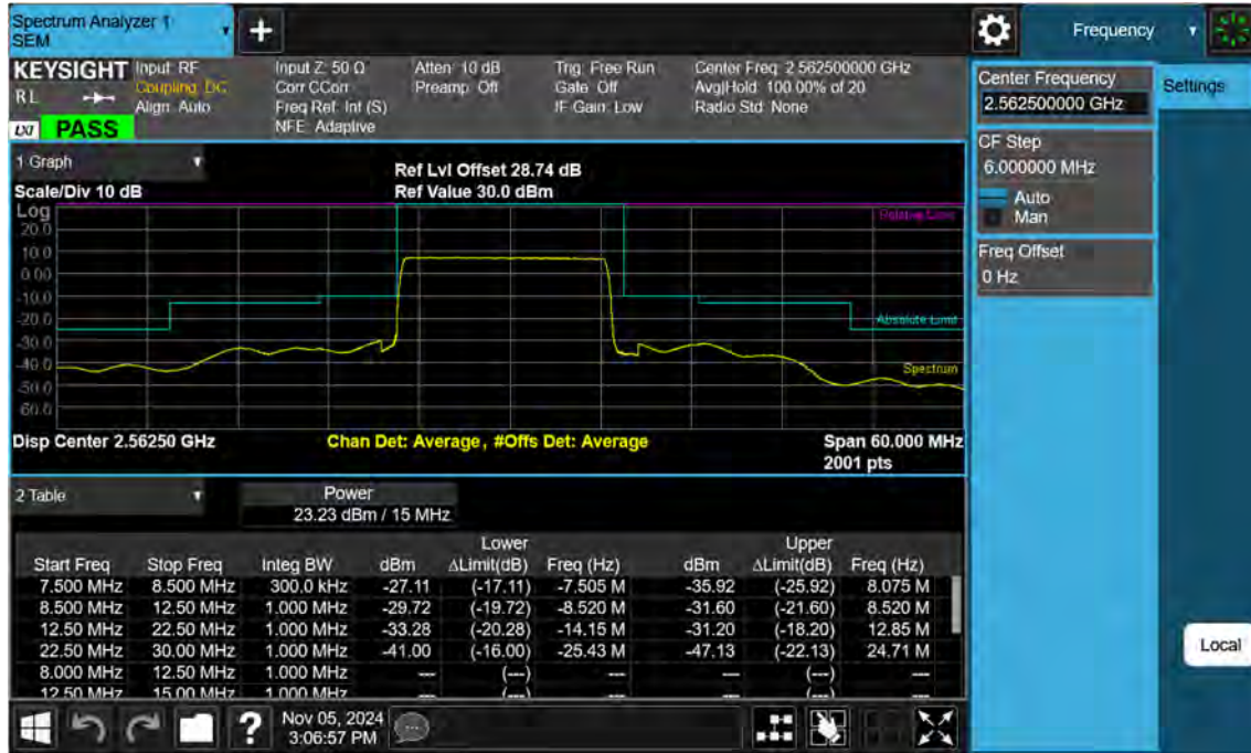
Sub6 n7. High Channel Edge Plot (15 MHz Ch.512500 BPSK)
