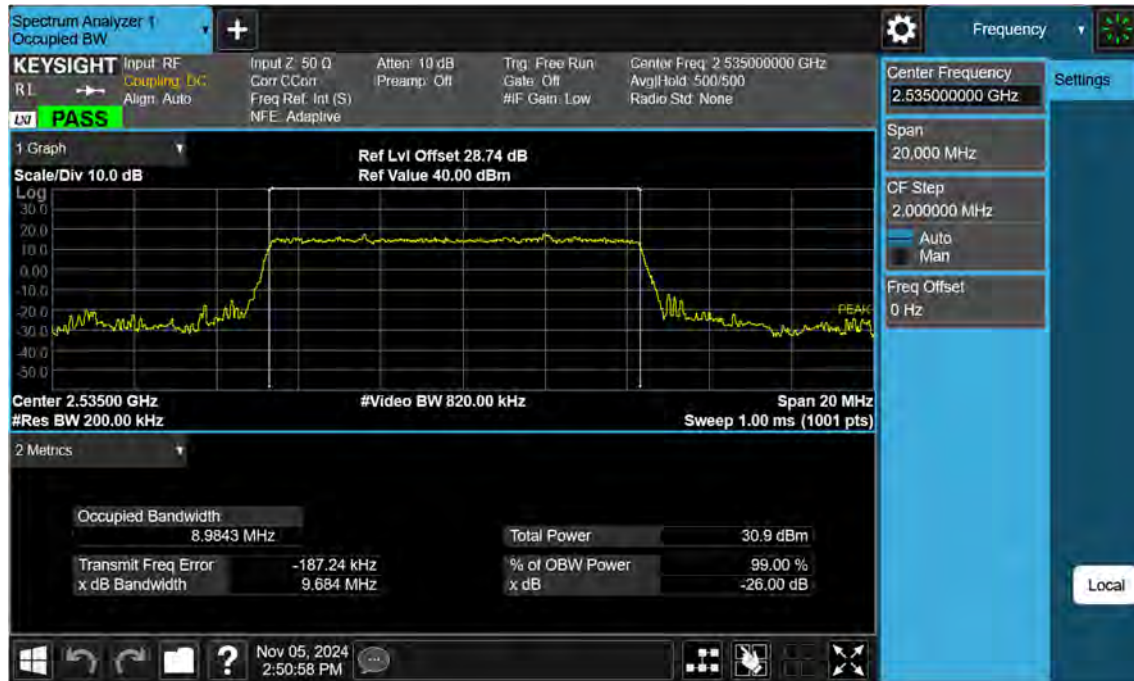
Sub6 n7. Occupied Bandwidth Plot (10 M BW Ch.507000 BPSK)
