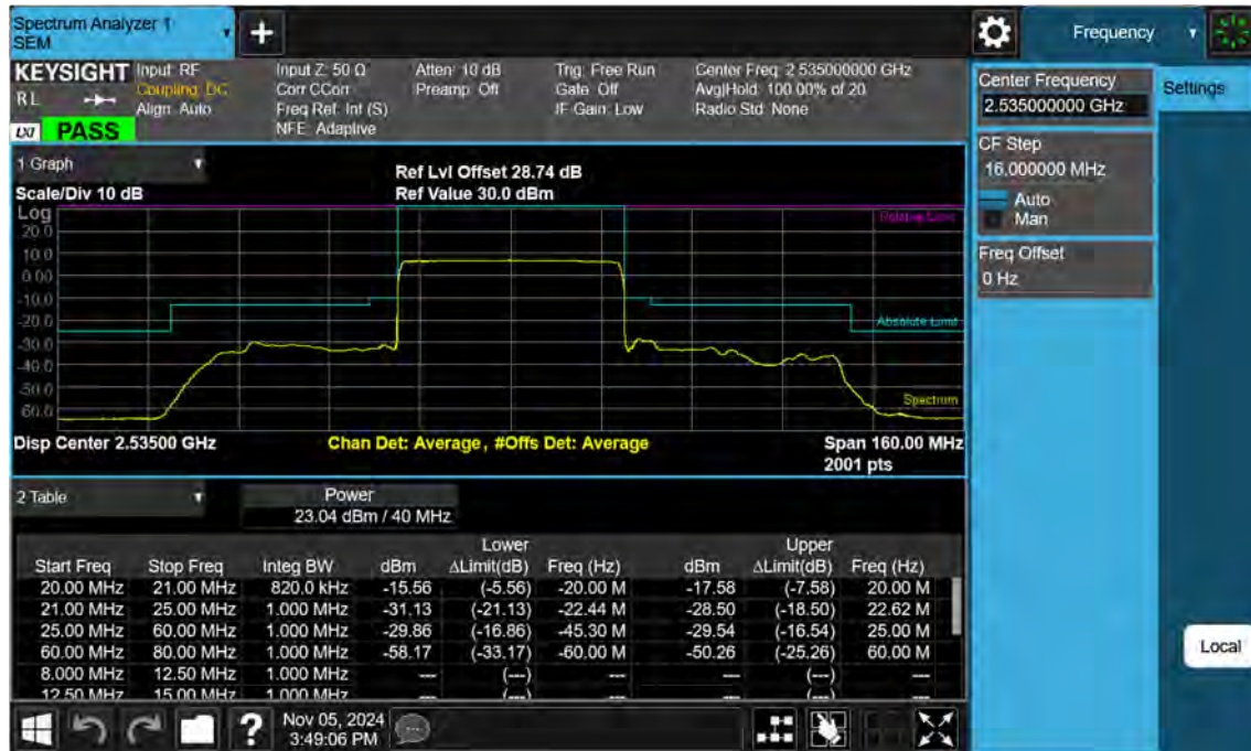
Sub6 n7. Mid Channel Edge Plot (40 MHz Ch.507000 BPSK)
