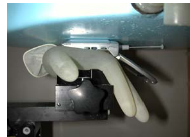
Figure 24. Hand SAR Test Setup
