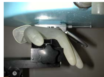
Figure 23. Hand SAR Test Setup
