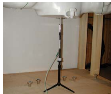
Figure 12.1 Dipole Validation Test Setup
