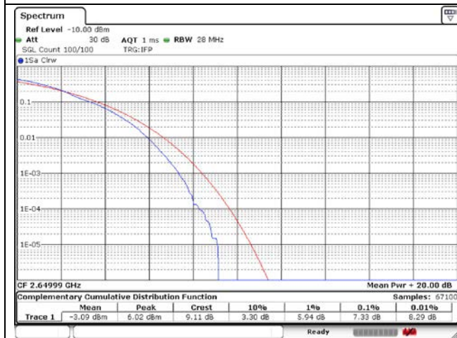
80 MHz High Channel - Full RB - DFT-S-OFDM
