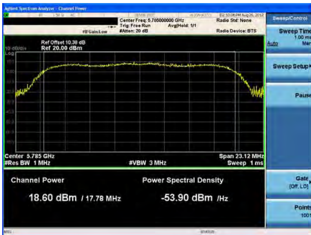
Conducted Output Power (802.11n-CH 157) 19.5 Mbps
