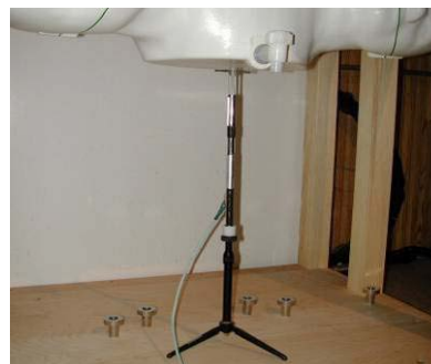
Figure 12-2 System Verification Setup Photo
