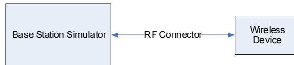
Figure 11-1 Power Measurement Setup
