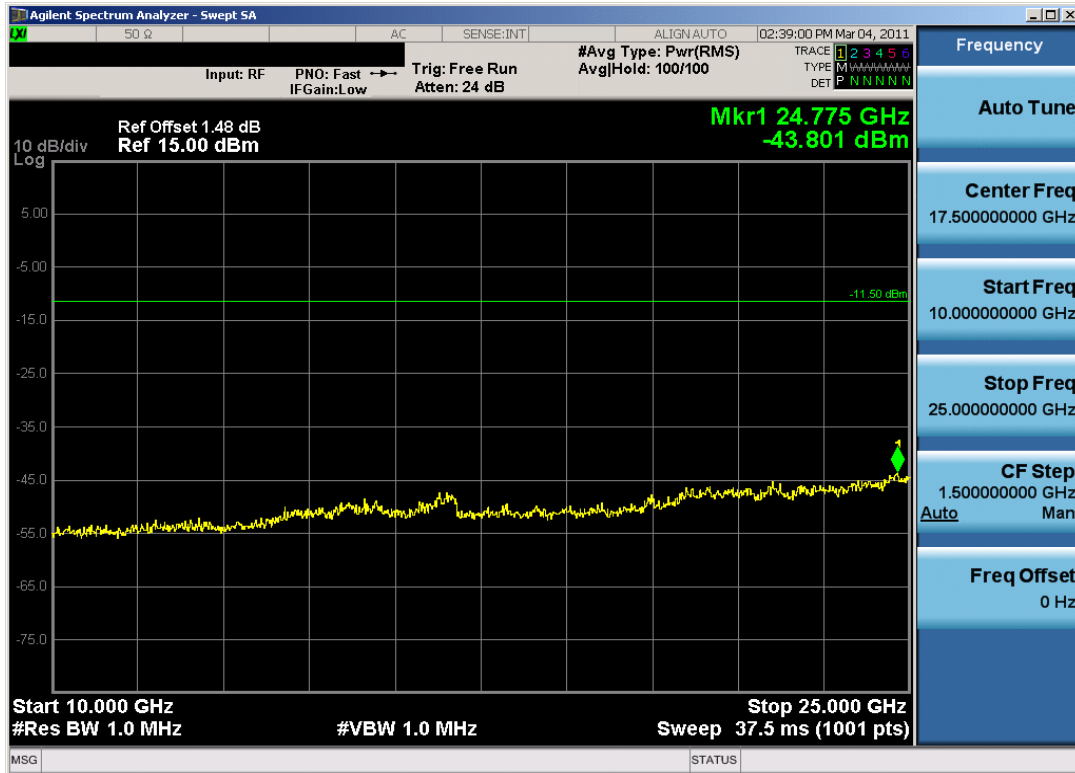
Plot 6-21. Conducted Spurious Plot (Bluetooth, 3Mbps – Ch. 39)
