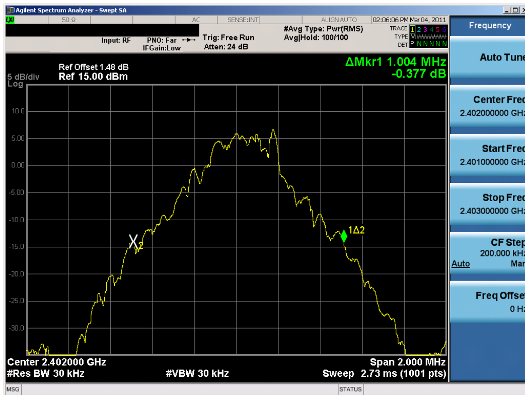
Plot 6-1. 20dB Bandwidth Plot (Bluetooth, 1Mbps - Ch. 0)
