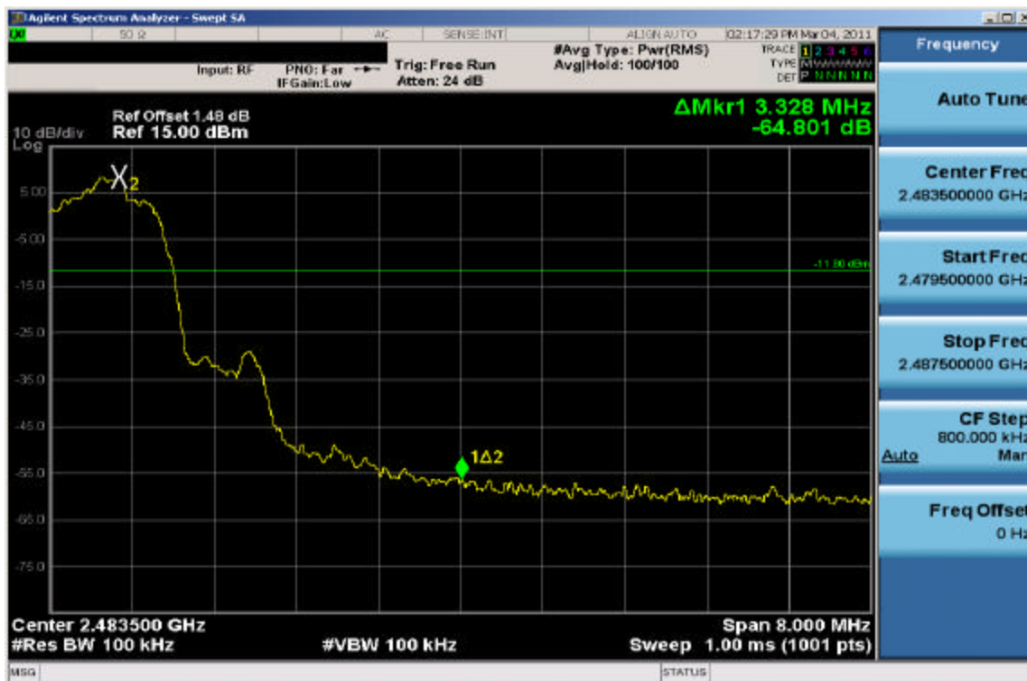
Plot 6-13. Band Edge Plot (Bluetooth, 3Mbps – Ch. 78)
