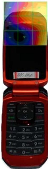
Figure 17-4 E-Field WD Scan overlay
