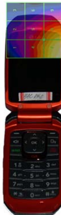
Figure 17-5 H-Field WD Scan overlay
