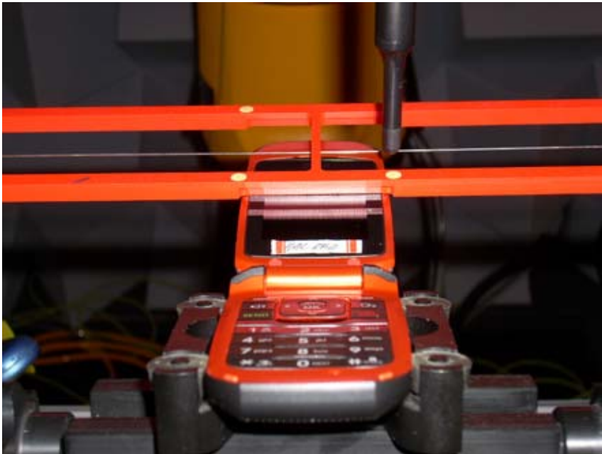
Figure 17-2 HAC Phantom Plane Alignment
