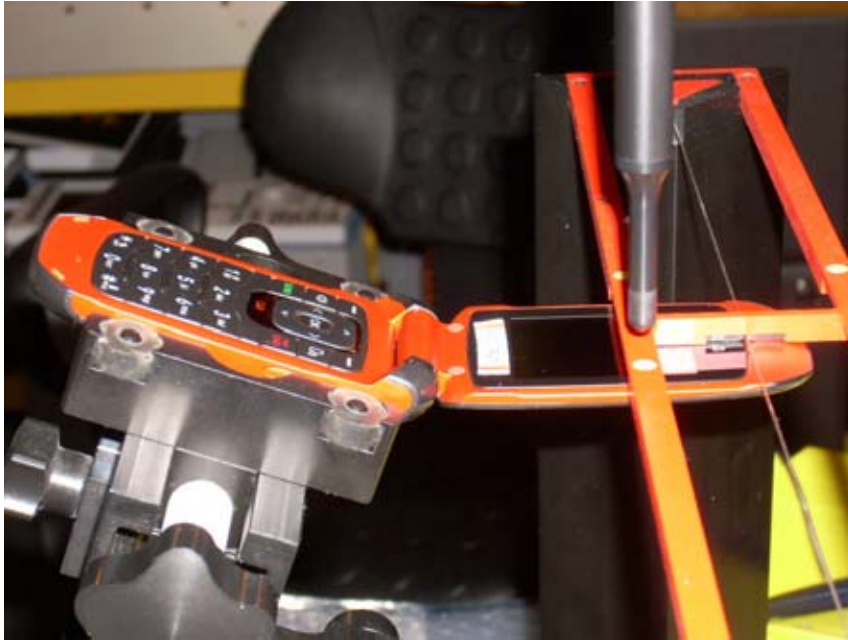
Figure 17-1 Ear Reference Point HAC Phantom Alignment
