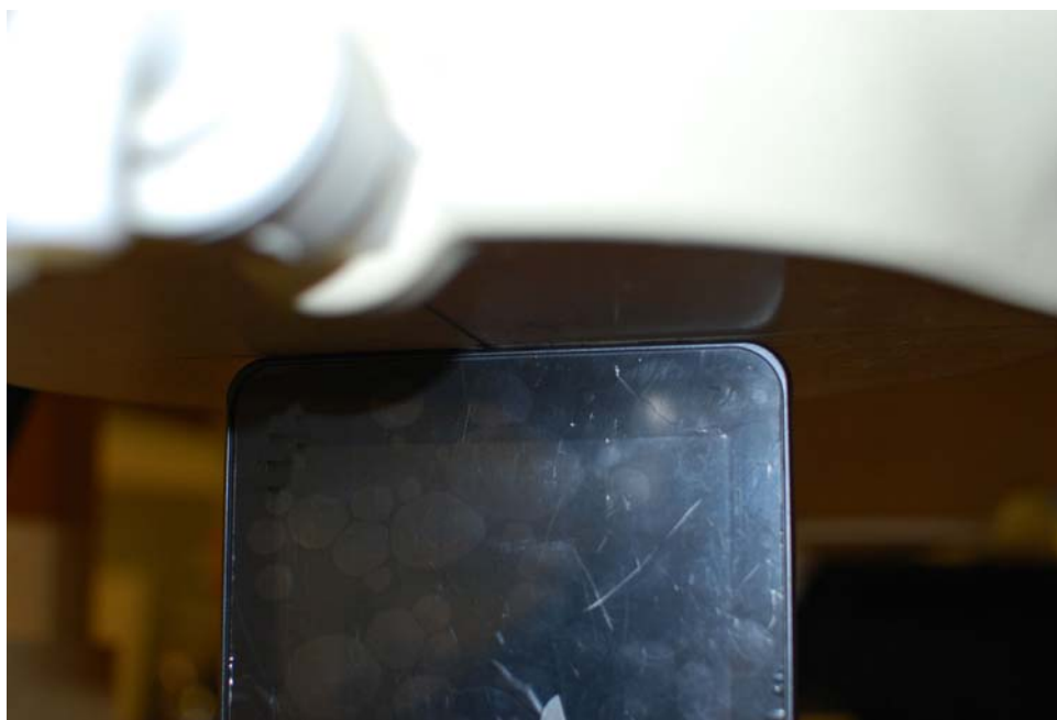
Figure 21-4 SAR Test Setup Photo 4: Top at 0.0 cm
