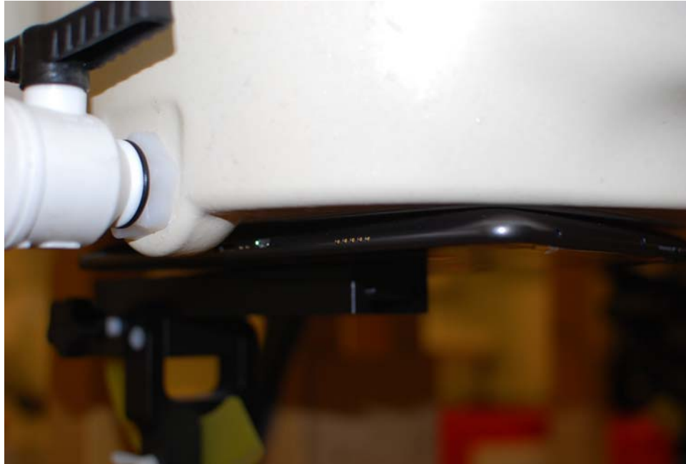
Figure 21-1 SAR Test Setup Photo 1: Back at 0.0 cm
