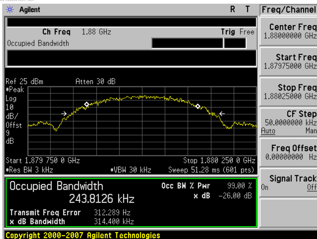
Plot 7-21. Occupied Bandwidth Plot (EDGE1900 Mode – Ch. 661)
