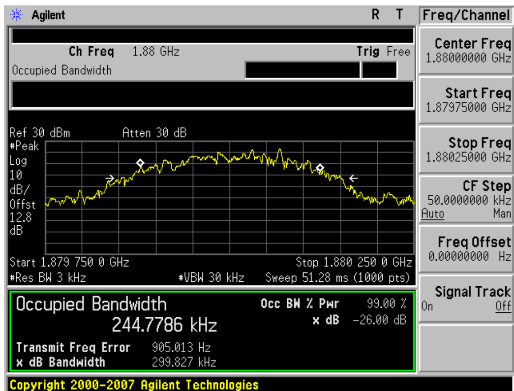
Plot 7-16. Occupied Bandwidth Plot (PCS GSM Mode – Ch. 661)
