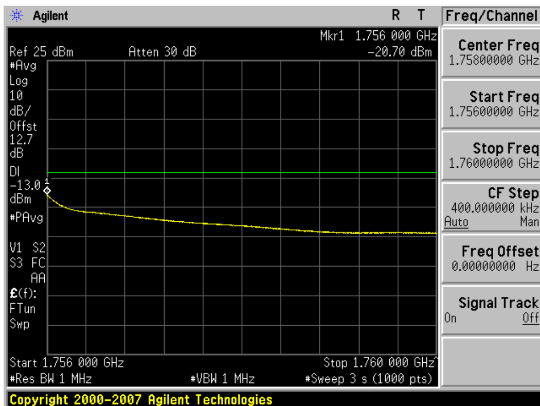
Plot 7-34. 4MHz Span Plot (AWS WCDMA Mode – Ch. 1862)
