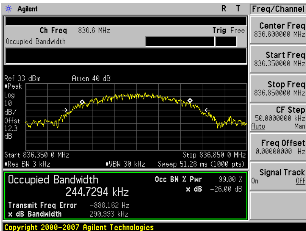
Plot 7-10. Occupied Bandwidth Plot (EDGE850 Mode – Ch. 190)
