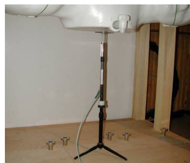
Figure 11-2 System Verification Setup Photo
