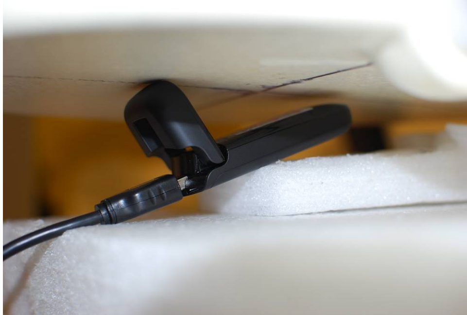
Figure 18-3 SAR Test Setup Photo 3 – Horizontal Down
