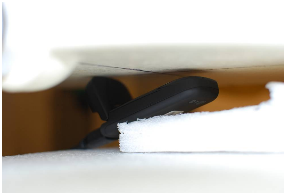
Figure 18-4 SAR Test Setup Photo 4 – Horizontal Down
