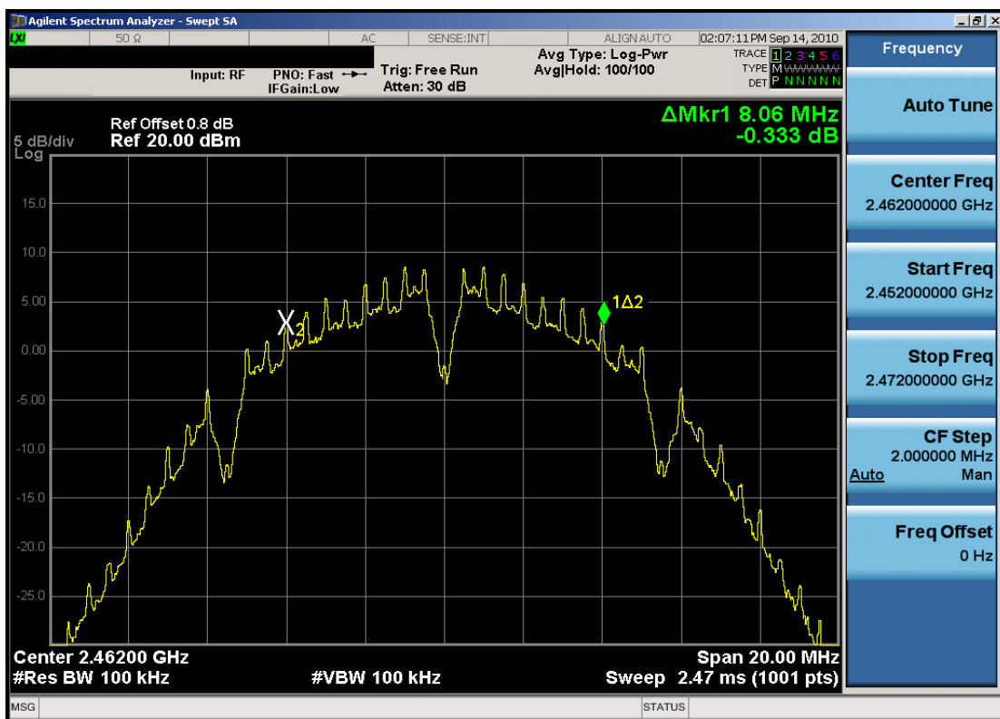
Plot 6-3. 6dB Bandwidth Plot (802.11b – Ch. 11)
