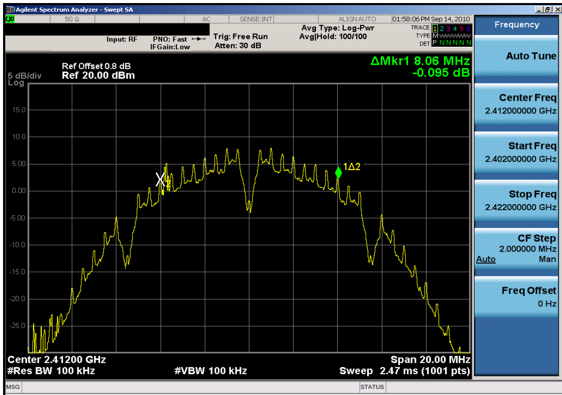
Plot 6-1. 6dB Bandwidth Plot (802.11b - Ch. 1)
