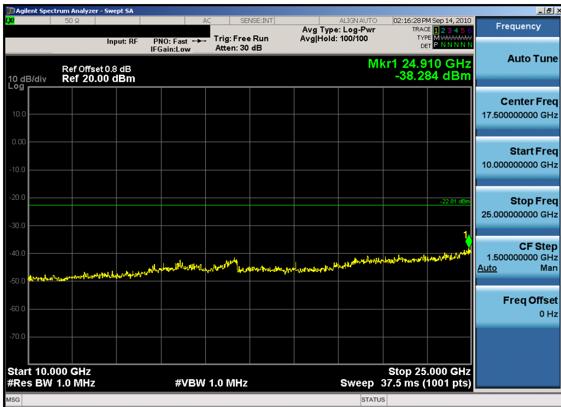
Plot 6-12. Conducted Spurious Plot (802.11b - Ch. 1)
