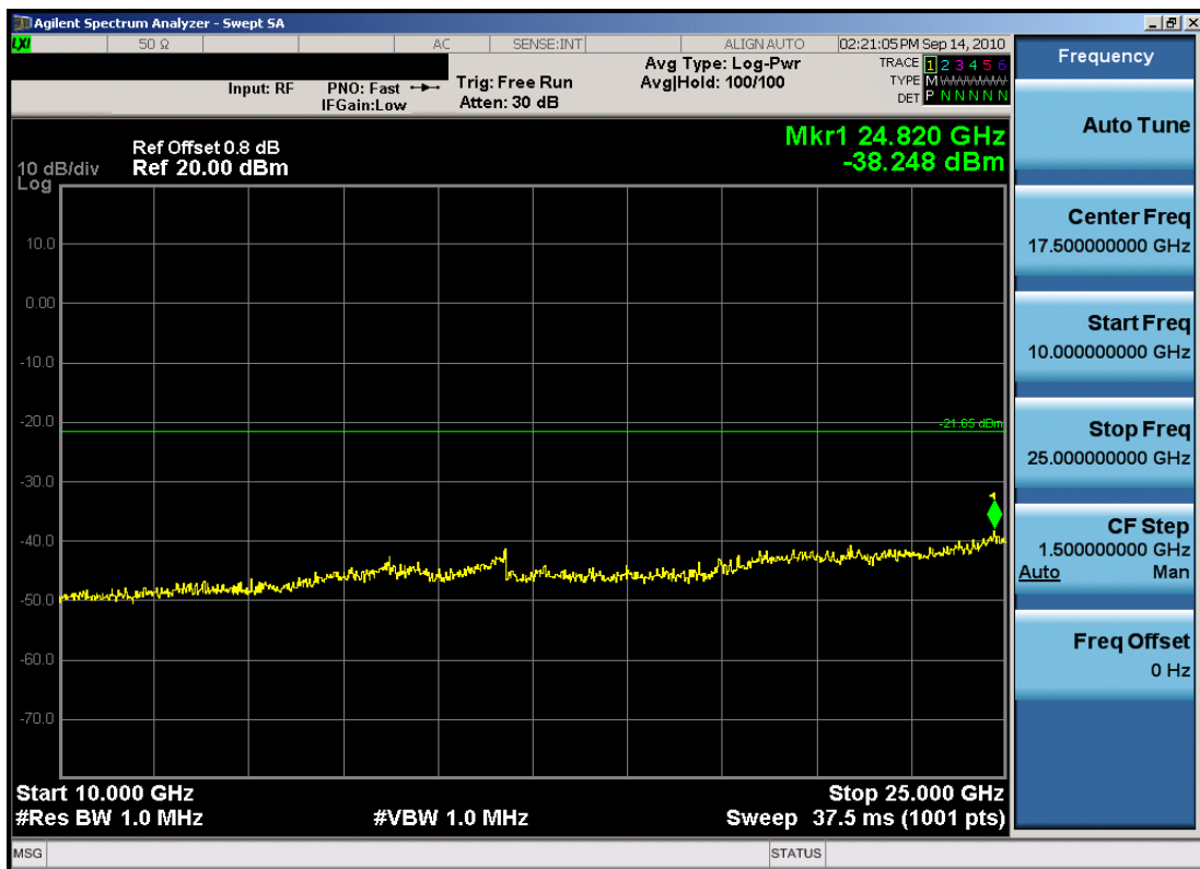
Plot 6-16. Conducted Spurious Plot (802.11b – Ch. 11)
