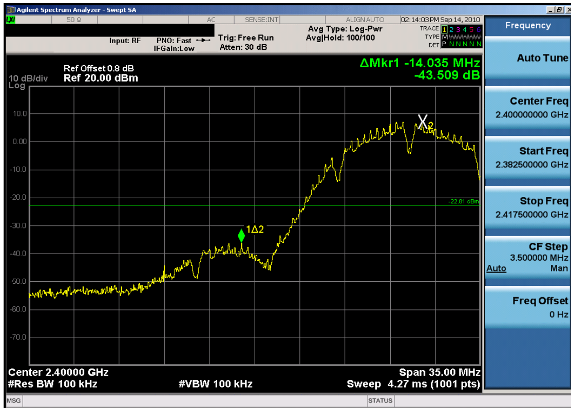
Plot 6-7. Band Edge Plot (802.11b – Ch. 1)
