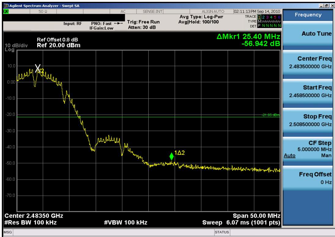
Plot 6-8. Band Edge Plot (802.11b – Ch. 11)
