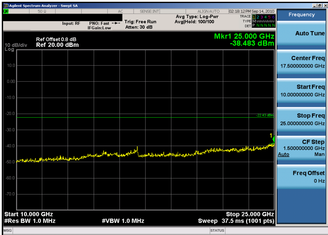
Plot 6-14. Conducted Spurious Plot (802.11b – Ch. 6)
