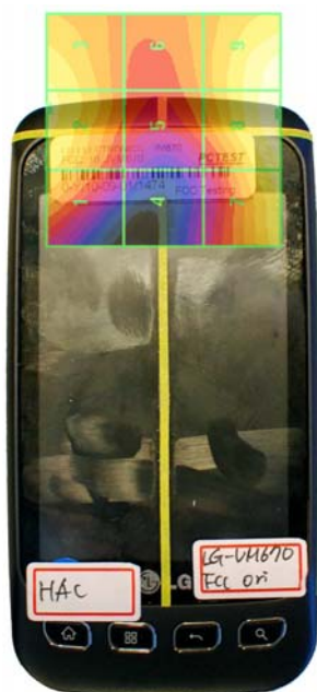
Figure 17-4 E-Field WD Scan overlay
