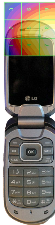
Figure 17-5 H-Field WD Scan overlay
