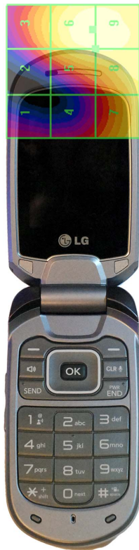
Figure 17-4 E-Field WD Scan overlay
