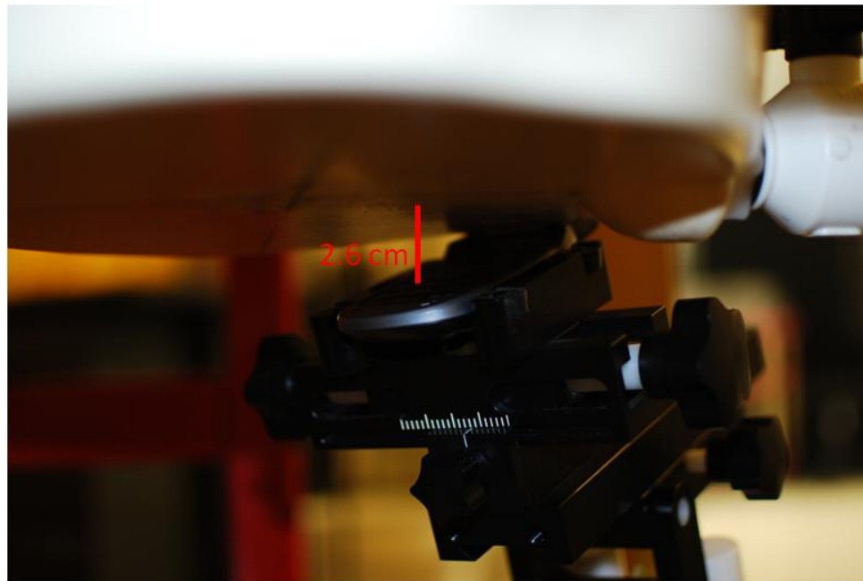
Figure 19-2 SAR Test Setup Photo 4 – Mouth-Jaw 2.6 cm
