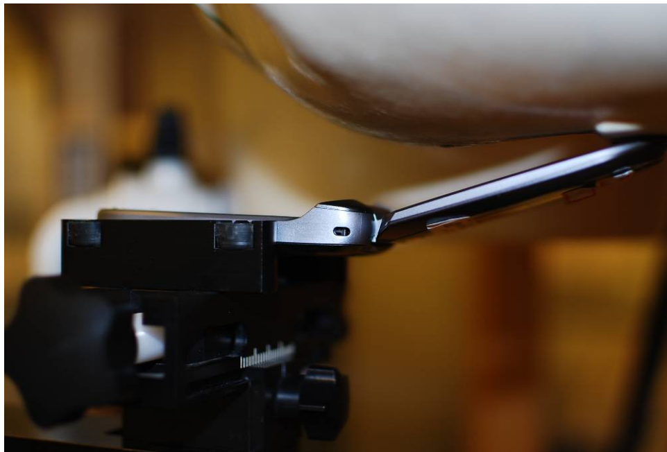
Figure 19-4 SAR Test Setup Photo 2 – Left Tilt
