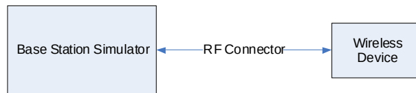
Figure 14-1 Power Measurement Setup
