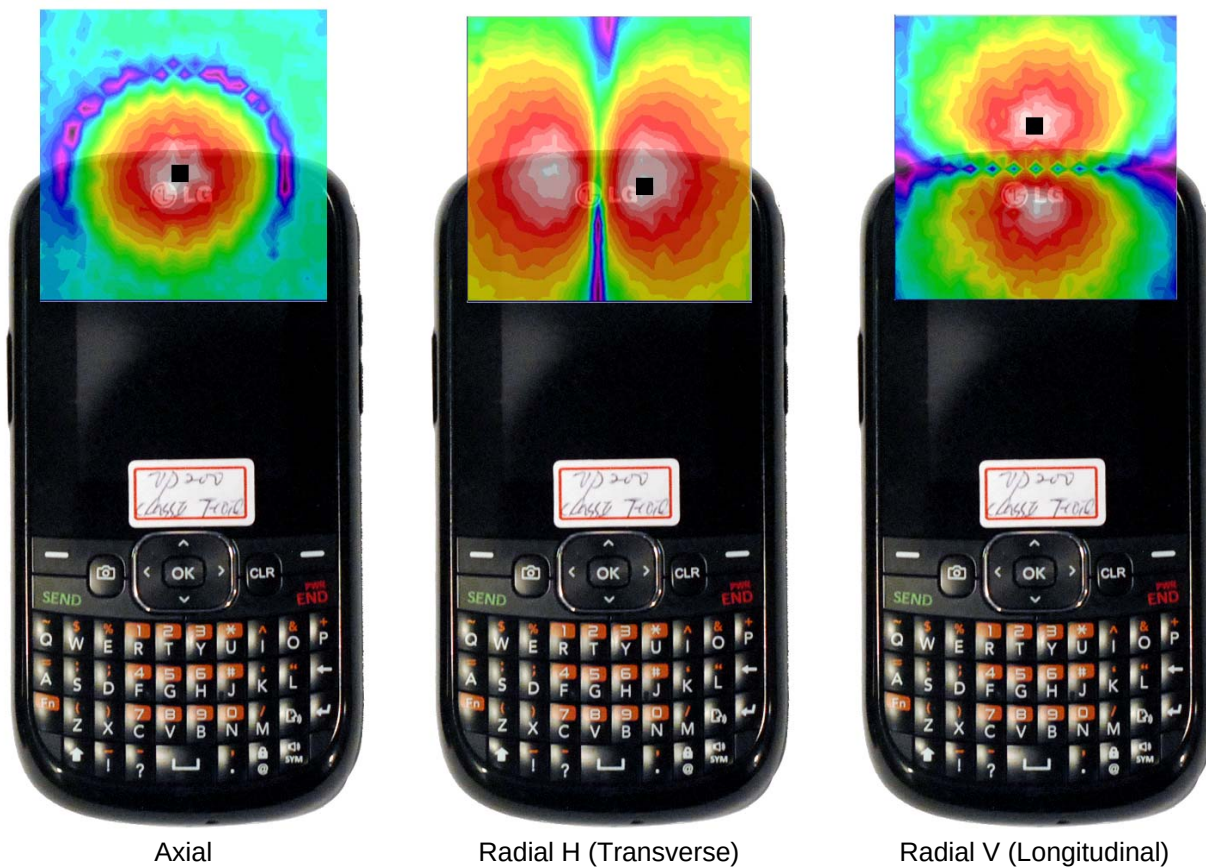
Figure 13-3 T-Coil Scan Overlay Magnetic Field Distributions
