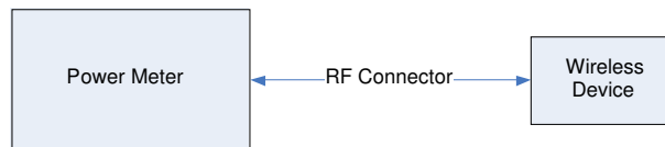
Figure 15-1 Power Measurement Setup
