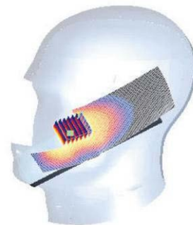
Figure 7-1 Sample SAR Area Scan
