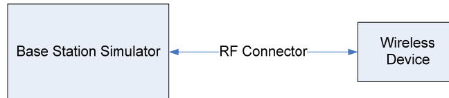
Figure 9-1 Power Measurement Setup
