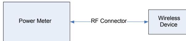
Figure 12-1 Power Measurement Setup
