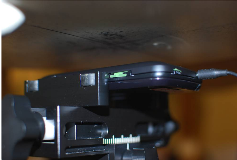
SAR Test Setup Photo 11 – Body Back at 2.0 cm
