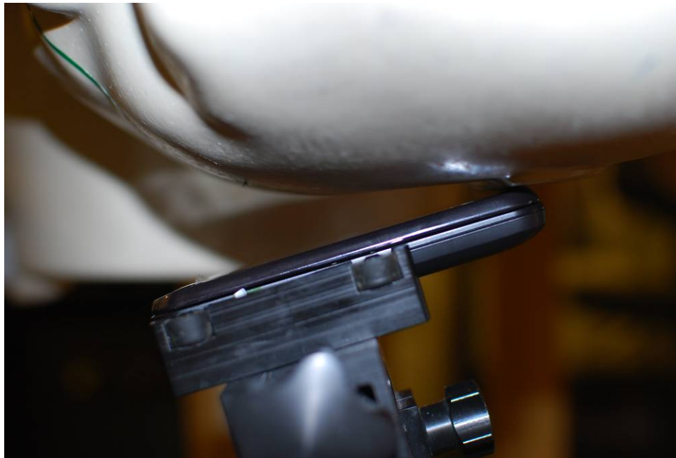
SAR Test Setup Photo 4 – Left Tilt
