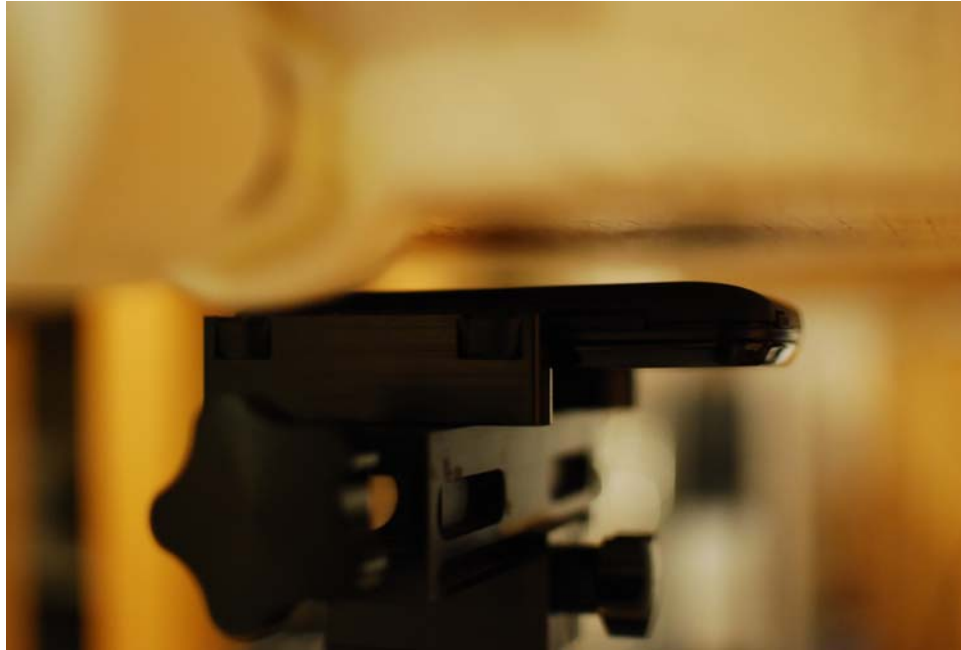
SAR Test Setup Photo 5: Back at 1.0 cm
