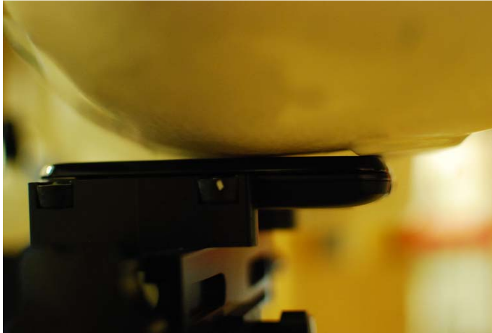
SAR Test Setup Photo 3: Left Touch
