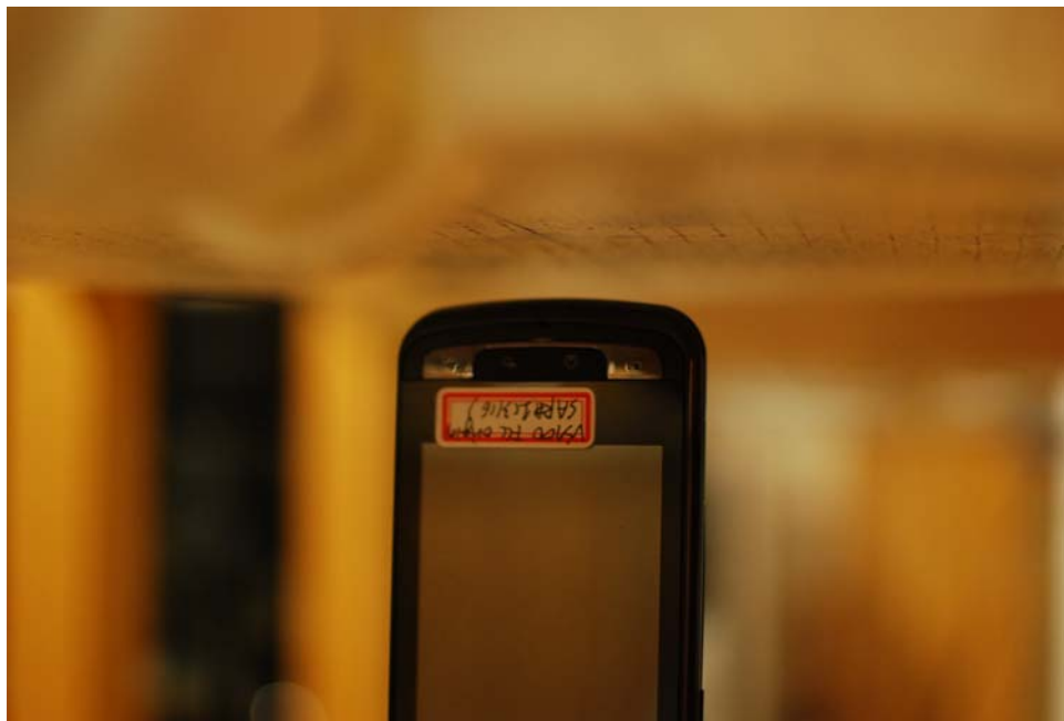
SAR Test Setup Photo 8: Bottom at 1.0 cm
