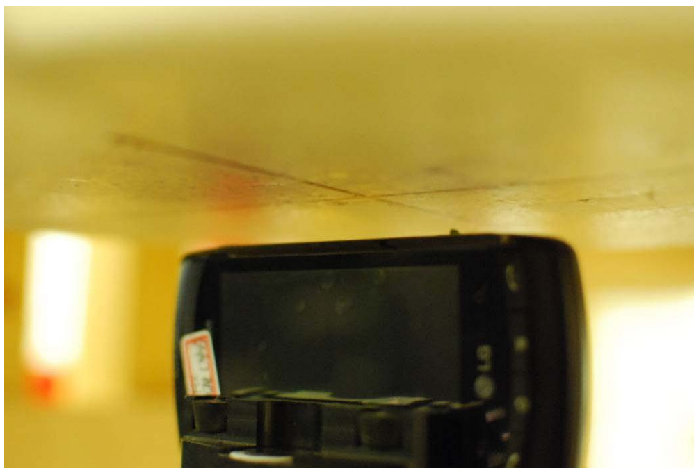
Figure 19-5 SAR Test Setup Photo 5 – Right at 1.0 cm
