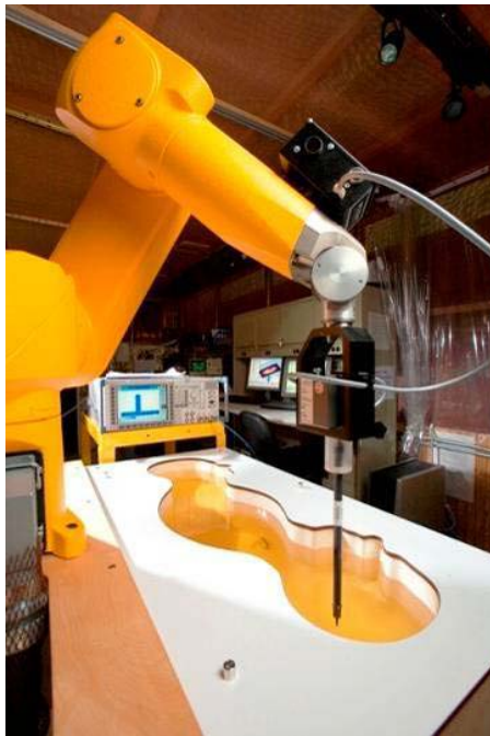
Figure 3-2 SAR Measurement System
