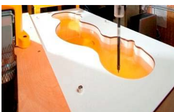
Figure 6-2 SAM Phantom with Simulating Tissue
