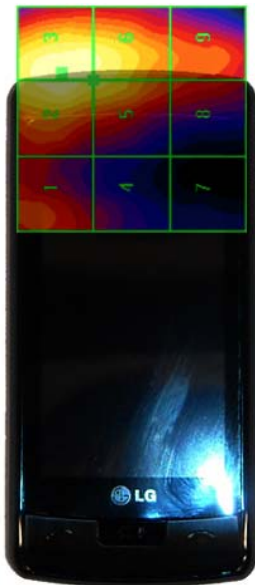
Figure 17-4 E-Field WD Scan overlay
