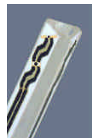
Figure 3.2 Probe Thick-Film Technique
