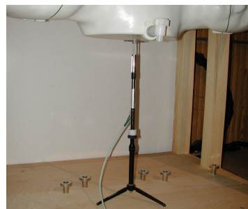
Figure 12.1 Dipole Validation Test Setup
