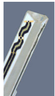
Figure 3.2 Probe Thick-Film Technique
