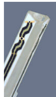
Figure 3.2 Probe Thick-Film Technique
