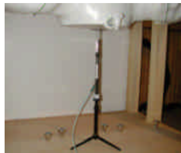
Figure 12.1 Dipole Validation Test Setup
