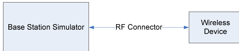
Figure 14-1 Power Measurement Setup
